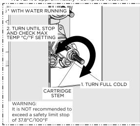
17. Re-open the DIVERTER VALVE then turn the THERMOSTATIC CARTRIDGE STEM clockwise to full cold then counterclockwise until it stops. Verify the **maximum** desired bathing temperature set in the previous step then turn the water off.
