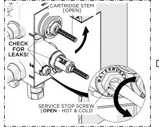
13. **OPEN** the SERVICE STOPS (hot & cold) and check for leaks.
