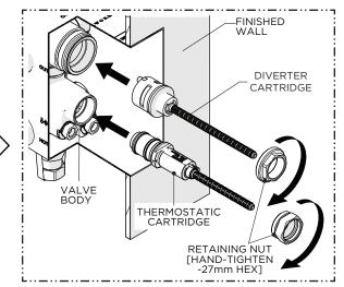
4. Insert the THERMOSTATIC CARTRIDGE and DIVERTER CARTRIDGE into the VALVE BODY then thread and hand-tighten the RETAINING NUTS into the VALVE BODY.
