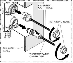
9. Unthread both RETAINING NUTS and remove both CARTRIDGES.
