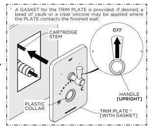
20. With the DIVERTER HANDLE in an upright vertical position, slide the HANDLE onto the CARTRIDGE STEM.
