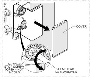
Turn on the water supplies then remove the COVER from the ViaBox™ and **OPEN** the SERVICE STOPS (hot & cold) to flush out the lines.
