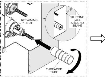
19. Thread the THREADED TUBE back into the RETAINING NUT until snug.
