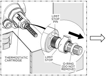
12. Slide the O-RING and LIMIT STOP on the THERMOSTATIC CARTRIDGE up the STEM.
