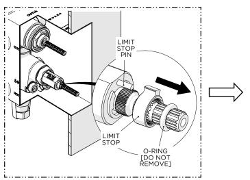
IF THE MAXIMUM BATHING TEMPERATURE IS NOT CORRECT OR NEEDS TO BE ADJUSTED:
