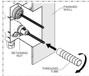
5. Thread the THREADED TUBE THERMOSTATIC RETAINING NUT until snug.
