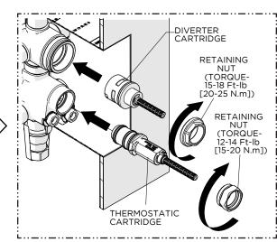
11. Insert both CARTRIDGES back into the VALVE BODY then thread and securely tighten the RETAINING NUTS to the specified torque settings shown.
