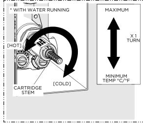
14. With water running, slowly rotate the THERMOSTATIC CARTRIDGE STEM clockwise to attain full cold then rotate it counterclockwise to attain full hot. Verify that a full range of temperatures exists.
