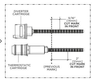
10. Carefully cut the DIVERTER STEM 9/16" [14mm] in front of the previous mark and THERMOSTATIC STEM 2" [51mm] in front of the previous mark so the STEMS will protrude 9/16" [14mm] and 2" [51mm] from the finished wall surface respectively.
