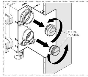
3. Unthread and remove the FLUSH PLATES. NOTE: Do NOT discard the FLUSH PLATES.
