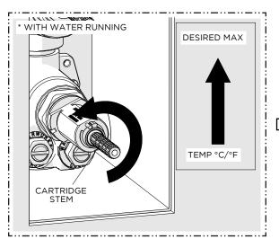
15. Rotate the THERMOSTATIC CARTRIDGE STEM to adjust the temperature to the maximum desired bathing temperature, verified with a thermometer, then close the DIVERTER VALVE and make sure NOT to change this setting.
