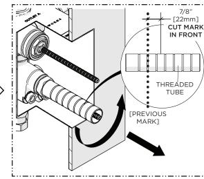
7. Remove the TUBE and cut it 7/8" [22mm] in front of the previous mark so the TUBE will protrude 7/8" [22mm] from the finished wall surface.
