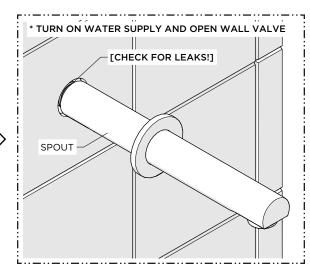
Turn on the water supply and open a diverter/ wall valve (sold separately) to flush out any debris in the supply line and inspect all connections for leaks.
