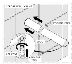
Close the diverter/wall valve then re-install the AERATOR and CAREFULLY slide the ESCUTCHEON down the SPOUT until it contacts the finished wall.
