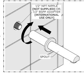
Thread and securely tighten the SPOUT onto the NPT NIPPLE or BSPP ADAPTER.
