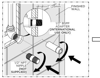
1. Install a 1/2" NPT NIPPLE (not supplied) and ensure it protrudes 1" [25mm] from the finished wall.
