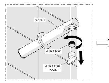
4. Using the TOOL provided, remove the AERATOR.
