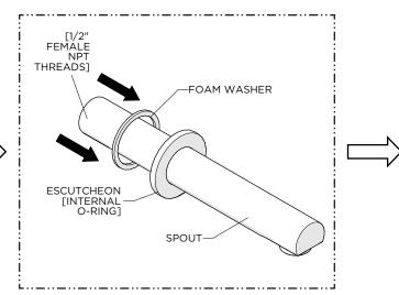
CAREFULLY slide the ESCUTCHEON and FOAM WASHER down the SPOUT.
