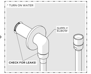
9. Turn on the water and a diverter/wall valve (sold separately) to flush out any debris in the supply line and inspect all connections for leaks then turn the water off.
