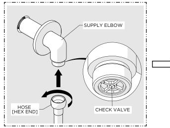
8. Thread and securely tighten the HEX end of the HOSE to the SUPPLY ELBOW.
