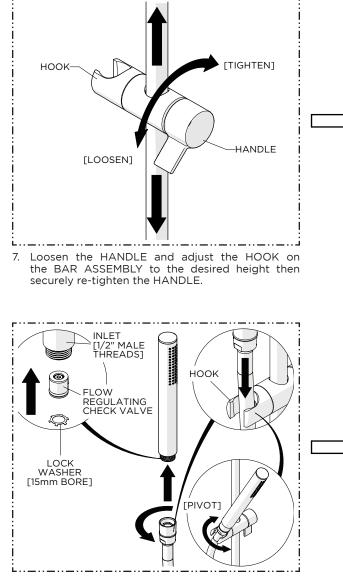
10. Thread and securely tighten the conical end of the HOSE to the HANDSHOWER then place it into the HOOK and pivot the HANDSHOWER to the desired position.
