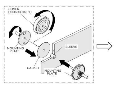
3. Insert the SLEEVE into the pre-drilled hole, insert the SET SCREW through the SLEEVE, and slide the second GASKET onto the SCREW then thread the COVER, or second MOUNTING PLATE, onto the SCREW.
