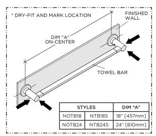
Dry-fit the TOWEL BAR to the finished wall and mark the ideal location making sure to hold the BAR level.
