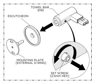
Loosen, but do NOT remove, the SET SCREW on the bottom of each TOWEL BAR END and remove the MOUNTING PLATES and ESCUTCHEONS.
