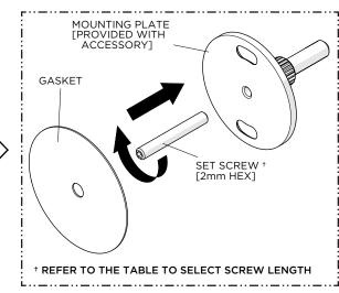
Thread the appropriate length SET SCREW into the MOUNTING PLATE then slide the GASKET over the SCRFW.
