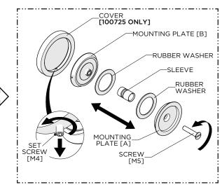
Disassemble the components by unthreading the SCREW on the MOUNTING PLATE [A].
