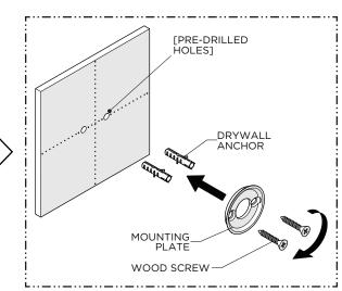
Using the previous marks as a reference, install the MOUNTING PLATE using the SCREWS and ANCHORS provided.
