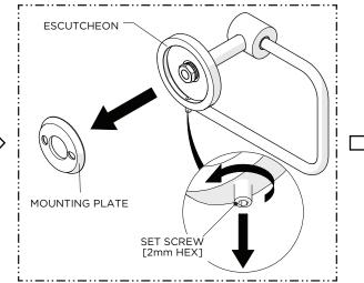
Loosen, but do NOT remove, the SET SCREW on the bottom of the ESCUTCHEON using a 2mm HEX KEY then remove the MOUNTING PLATE.
