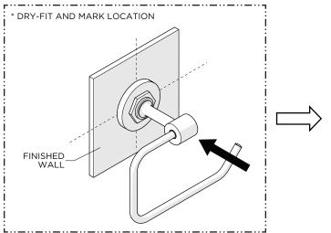
Dry-fit the product to the finished wall and mark the ideal location for installation.
