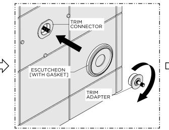
13. Hold the ESCUTCHEON against the finished wall then thread the TRIM ADAPTER into the TRIM CONNECTOR until snug.
