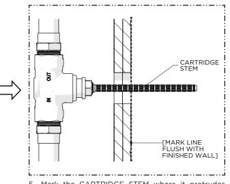
5. Mark the CARTRIDGE STEM where it protrudes past the finished wall.
