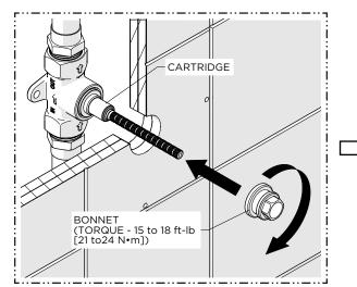
12. Remove the HANDLE then thread and securely tighten the BONNET back onto the CARTRIDGE.
