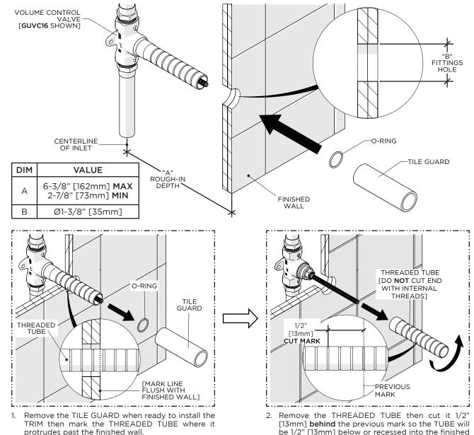
NOTE: A straight edge (not supplied) can be used to mark the TUBE.
