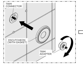
15. Hold the ESCUTCHEON against the finished wall then thread the TRIM ADAPTER into the TRIM CONNECTOR until snug.
