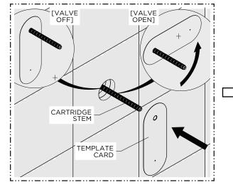
3. With the VALVE in the off position, slide the TEMPLATE onto the STEM. Mark the 1st PIN HOLE location then rotate the STEM to the full open position and mark the 2nd hole location.
