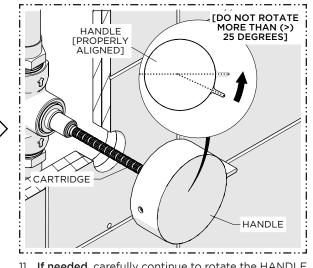
If needed, carefully continue to rotate the HANDLE counter-clockwise to obtain the proper alignment. Do NOT rotate/unthread the CARTRIDGE more than 25 degrees.
