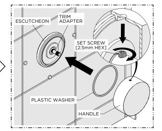
14. Slide the PLASTIC WASHER onto the ESCUTCHEON then place the HANDLE onto the TRIM ADAPTER. Ensure the HANDLE is fully seated and properly aligned with the PINS then thread and securely tighten the SET SCREW.
