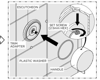
16. Slide the PLASTIC WASHER onto the ESCUTCHEON then place the HANDLE onto the TRIM ADAPTER. Ensure the HANDLE is fully seated and properly aligned with the PINS then thread and securely tighten the SET SCREW.
