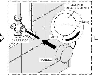
10. Remove and replace the HANDLE and TRIM ADAPTER to position them as close as possible to the "OFF" position then turn the HANDLE a 1/4 turn to the "OPEN" position making sure NOT to unthread the CARTRIDGE.
