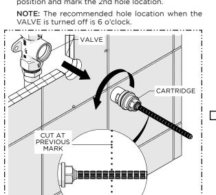
Remove the CARTRIDGE using a 21/32" [17mm] shower valve socket wrench (not supplied) then cut the CARTRIDGE STEM at the previous mark.
