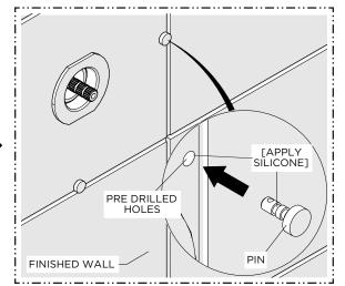
14. A SILICONE SEALANT is provided. Apply an appropriate amount of SEALANT into the predrilled holes and the PINS then insert the PINS into the holes until flush with the finished wall. Wipe away any excess SEALANT.
