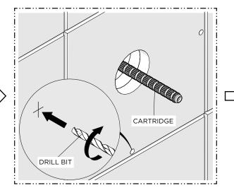
4. Using the previous marks as a reference, carefully drill the holes into the finished wall using the DRILL BIT provided.
