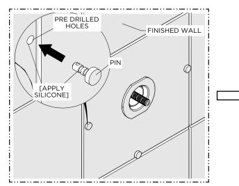
12. A SILICONE SEALANT is provided. Apply an appropriate amount of SEALANT into the predrilled holes and the PINS then insert the PINS into the holes until flush with the finished wall. Wipe away any excess SEALANT.
