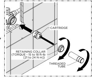
10. Re-insert the CARTRIDGE then thread and securely tighten the RETAINING COLLAR to the specified torque setting shown.
