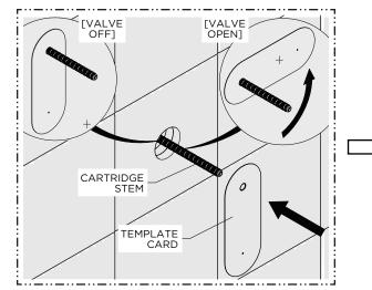
3. Slide the TEMPLATE onto the STEM at the 3 o'clock position. Mark the 1st PIN HOLE location then rotate the STEM through the various VALVE positions and mark the additional hole locations.
