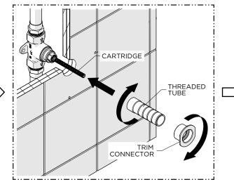
13. Thread and securely tighten the THREADED TUBE back onto the CARTRIDGE until snug then thread the TRIM CONNECTOR onto the THREADED TUBE until snug.
