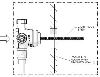
Mark the CARTRIDGE STEM where it protrudes past the finished wall.
