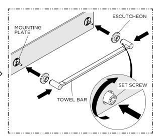
4. Slide the ESCUTCHEONS over the MOUNTING PLATES making sure they are fully seated. While holding the ENDS and BAR together, place both ENDS over the MOUNTING PLATES and into the ESCUTCHEON. Once fully seated, securely tighten the SET SCREWS.
