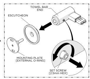
Loosen, but do NOT remove, the SET SCREW on the bottom of each TOWEL BAR END and remove the MOUNTING PLATES and ESCUTCHEONS.
