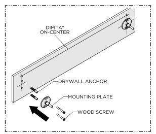
Using the previous marks as a reference, install the MOUNTING PLATES using the SCREWS and ANCHORS provided.
