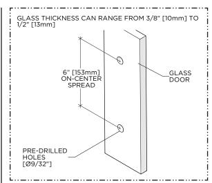
Drill two 9/32" [7mm] diameter holes on the mounting surface at the required on-center spread of 6" [152mm].
