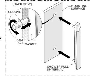
Using the GASKET provided, insert the POSTS on the SHOWER PULL (A) into the pre-drilled holes.
