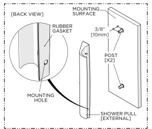
Using the GASKET provided, slide the SHOWER PULL (B) onto the POSTS until it contacts the mounting surface.
