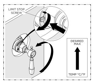
Open the VALVE to the maximum desired bathing temperature verified with a thermometer then turn the LIMIT STOP SCREW clockwise until it seats. Turn the VALVE off then on and verify the temperature previously set.
