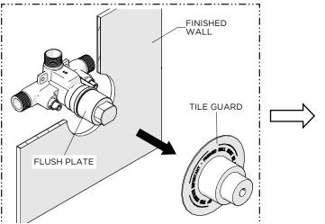
1. Remove the TILE GUARD from the VALVE when the TRIM is ready to be installed.
