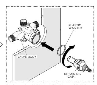
5. Using the PLASTIC WASHER provided, insert the CARTRIDGE into the VALVE then thread and securely tighten the RETAINING CAP.
