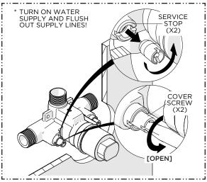
2. Turn on the water supplies then remove the COVER SCREWS (X2) and OPEN the SERVICE STOPS (X2) (hot & cold) to flush out the supply lines.
