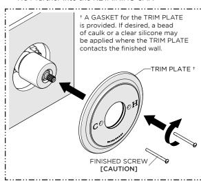
11. Slide the TRIM PLATE over the GLAND COVER then thread and securely tighten the SCREWS(X2).
