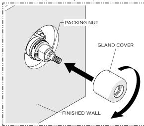
Thread and securely tighten the GLAND COVER onto the VALVE.
