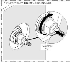
The PACKING NUT needs to be securely tightened to prevent a water leak from the CARTRIDGE STEM and create adequate rotational friction to maintain HANDLE position.
