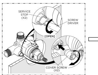
OPEN the SERVICE STOPS (hot & cold) then reinstall the COVER SCREWS (x2).
