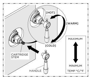
7. With the VALVE turned off, position the HANDLE on the CARTRIDGE STEM at the 6 o'clock position. Then, turn the HANDLE counterclockwise through the cold and warm settings, stopping at the hot position. Verify that a full range of temperatures exists.
