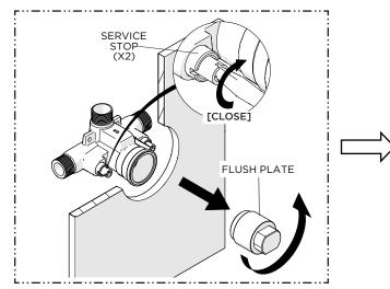
After the lines have been fully flushed, CLOSE the SERVICE STOPS (X2) (hot & cold) then unthread and remove the FLUSH PLATE.
