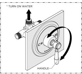
13. Turn on the water and operate the HANDLE to ensure it is functioning properly.
