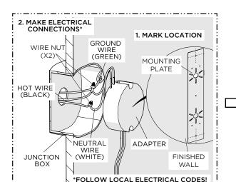
Dry fit and mark the screw locations on the finished wall. Use WIRE NUTS to connect the HOT (BLACK) and NEUTRAL (WHITE) wires.
