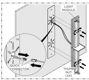
Connect the QUICK CONNECTOR from the ADAPTER to the QUICK CONNECTOR on the LIGHT MODULE. Position the LIGHT MODULE onto the MOUNTING PLATE ensuring the screw holes align. Fasten the THUMB NUTS to the LIGHT MODULE screws ensuring they are fully tightened.
