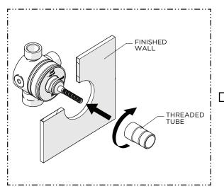
Thread the THREADED TUBE back onto the CARTRIDGE until it stops
