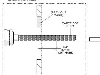
4. Carefully cut the CARTRIDGE STEM 1/4" [6mm] in front of the previous mark.
