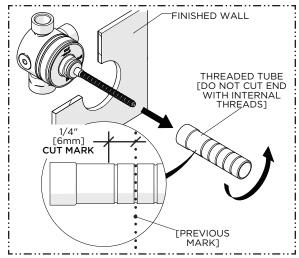
2. Remove the THREADED TUBE then cut it 1/4" [6mm] behind the previous mark.
