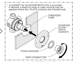
6. Firmly hold the DIVERTER PLATE against the finished wall then thread and securely tighten the TRIM CONNECTOR onto the THREADED TUBE making sure to use the FOAM WASHER provided.
