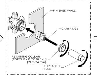
5. Re-insert the CARTRIDGE into the VALVE then thread and securely tighten the RETAINING COLLAR to the specified torque setting shown.
