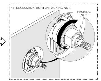
The PACKING NUT needs to be securely tightened to prevent a water leak from the CARTRIDGE STEM and create adequate rotational friction to maintain HANDLE position.
