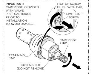
4. **IMPORTANT:** Leaving the PACKING NUT in place, unthread the LIMIT STOP SCREW until the O-RING is fully exposed then rotate the CARTRIDGE STEM counterclockwise to ensure the CARTRIDGE is drawn as close as possible to the RETAINING CAP.
