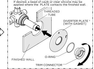
Firmly hold the DIVERTER PLATE against the finished wall then thread and securely tighten the TRIM CONNECTOR onto the THREADED TUBE making sure to use the O-RING provided.
