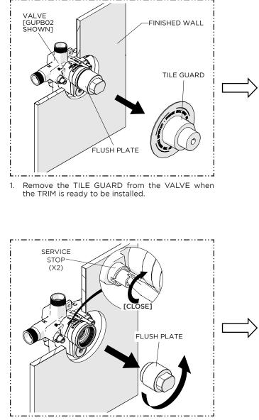
3. After the lines have been fully flushed, **CLOSE** the SERVICE STOPS (hot & cold) then unthread and remove the FLUSH PLATE.
