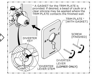
11. Slide the TRIM PLATE over the GLAND COVER then thread and securely tighten the SCREWS.
