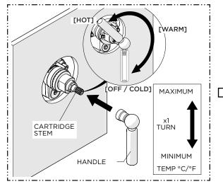
7. With the VALVE turned off, position the HANDLE on the CARTRIDGE STEM at the 6 o'clock position. Then, turn the HANDLE counterclockwise through the cold and warm settings, stopping at the hot position. Verify that a full range of temperatures exists.
