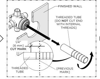
2. Remove the THREADED TUBE then cut it 1/4" [6 mm] **behind** the previous mark so the STEM will be 1/4" [6mm] below or recessed into the finished wall surface.
