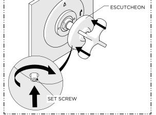
9. CAREFULLY slide the ESCUTCHEON down the HANDLE to conceal the TRIM CONNECTOR, then thread the SET SCREW to secure the position of the ESCUTCHEON.
