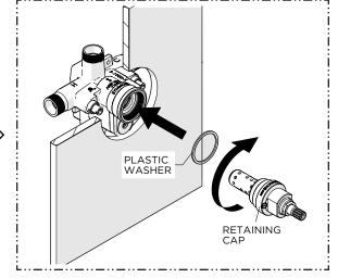
5. Using the PLASTIC WASHER provided, insert the CARTRIDGE into the VALVE then thread and securely tighten the RETAINING CAP.
