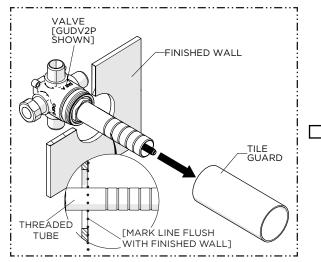
. Remove the TILE GUARD when ready to install the TRIM then mark the THREADED TUBE where it protrudes past the finished wall.
