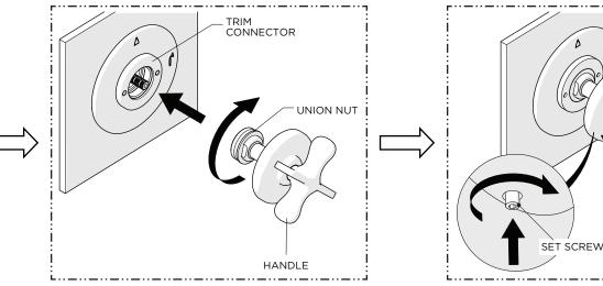
8. With the HANDLE in the desired orientation, thread the UNION NUT into the TRIM CONNECTOR until
