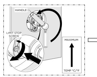
9. Open the VALVE to the **maximum** desired bathing temperature verified with a thermometer then turn the LIMIT STOP SCREW clockwise until it seats.
