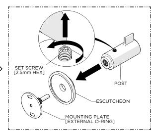
Loosen, but do NOT remove, the SET SCREW on the POST and remove the MOUNTING PLATE and ESCUTCHEON.
