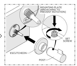
Slide the ESCUTCHEON and POST onto the MOUNTING PLATE then thread and securely tighten the SET SCREW.
