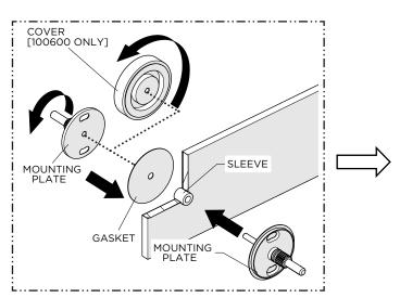
Insert the SLEEVE into the pre-drilled hole, insert the SET SCREW through the SLEEVE, and slide the second GASKET onto the SCREW then thread the COVER, or second MOUNTING PLATE, onto the SCREW.
