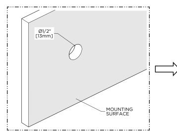
Ensure any pre-drilled hole is a 1/2" [13mm].
