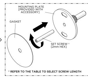
Thread the appropriate length SET SCREW into the MOUNTING PLATE then slide the GASKET over the SCREW.
