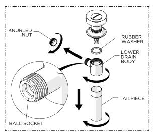
Remove the TAILPIECE and LOWER DRAIN BODY from the DRAIN FLANGE then remove the KNURLED NUT from the LOWER DRAIN BODY.
