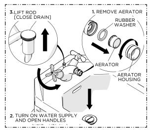
Remove the AERATOR then turn on the water supply and open the HANDLES to flush out the supply lines. Inspect all connections for leaks then close the DRAIN using the LIFT ROD to ensure it functions properly.
