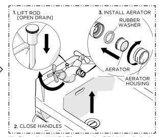
12. Close the HANDLES, open the DRAIN to drain the water, and re-install the AERATOR.
