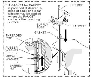
Insert the SUPPLY TUBES and THREADED ROD through the mounting hole using the GASKET PROVIDED. Attach the WASHERS onto the THREADED ROD, making sure not to obstruct the TUBES or LIFT ROD, then thread and securely tighten the BARREL NUT.
