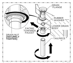
5. Using the WASHER provided, thread the LOWER DRAIN BODY back onto the FLANGE. Ensure the DRAIN BODY is positioned towards the FAUCET then securely tighten the DRAIN NUT. Ensure the GASKET makes a full seal on the underside of the BIDET. Thread and securely tighten the TAILPIECE back into the LOWER DRAIN BODY.
