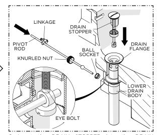
Insert the DRAIN STOPPER into the DRAIN FLANGE then insert the PIVOT ROD into the LOWER DRAIN BODY making sure the ROD passes through the EYEBOLT.
