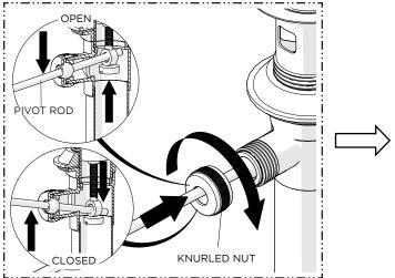
Ensure the PIVOT ROD opens and closes the DRAIN STOPPER properly, adjust the EYEBOLT if needed, then thread and securely tighten the KNURLED NUT.
