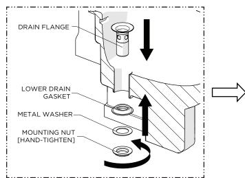
Set the DRAIN FLANGE into the BIDET (sold separately) using putty or a clear adhesive silicone. Re-attach the LOWER DRAIN GASKET and METAL WASHER then hand-tighten the MOUNTING NUT.
