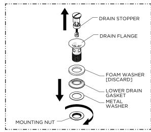
Remove the MOUNTING NUT, METAL WASHER, LOWER DRAIN GASKET and DRAIN STOPPER from the DRAIN FLANGE.
