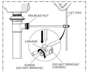
8. Insert the LIFT ROD through the hole in the LINKAGE then securely tighten the SCREW.
