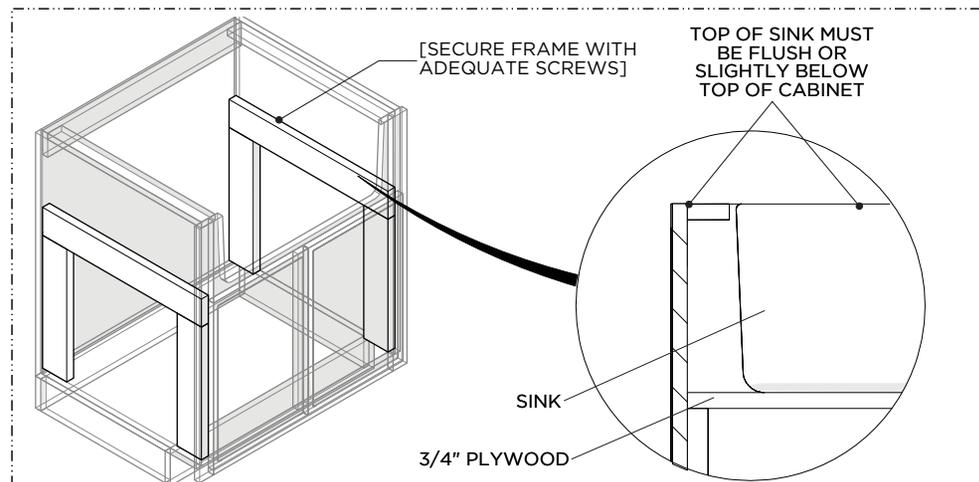
4. Ensure that the supports are secured using **SCREWS** (not provided) and level.
