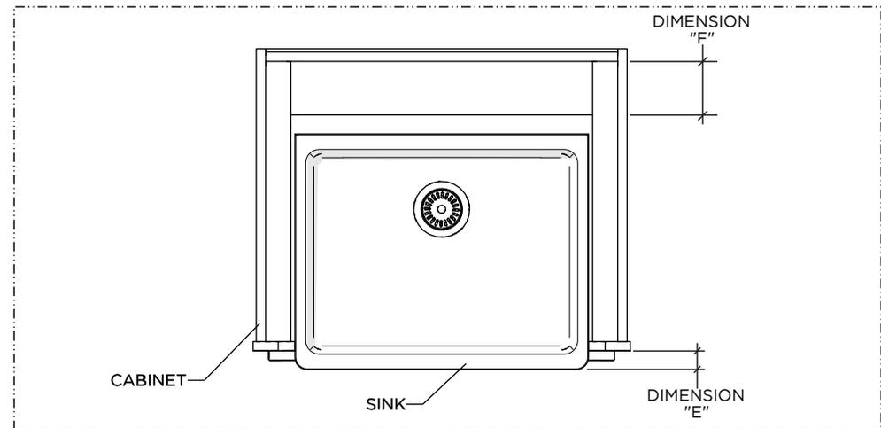
8. Position the SINK so that the apron or front of the SINK projects out of the cabinet as desired, **DIMENSION "E"**, and there is enough room between the SINK and the back of the cabinet, **DIMENSION "F"**, for the faucet fittings.
