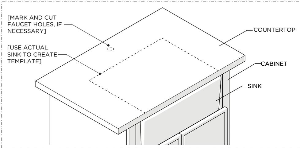
9. With the SINK in the final position, create a template to transfer onto the countertop then cut the countertop per manufacturer's instructions and cut the faucet hole(s) prior to final installation.
