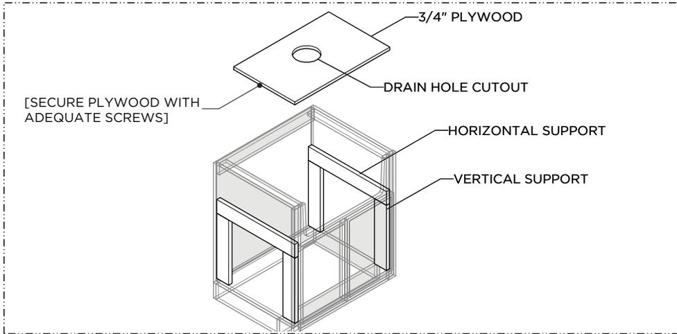
5. Cut out the portion of plywood for the drain connections then secure the plywood to the support framing.
