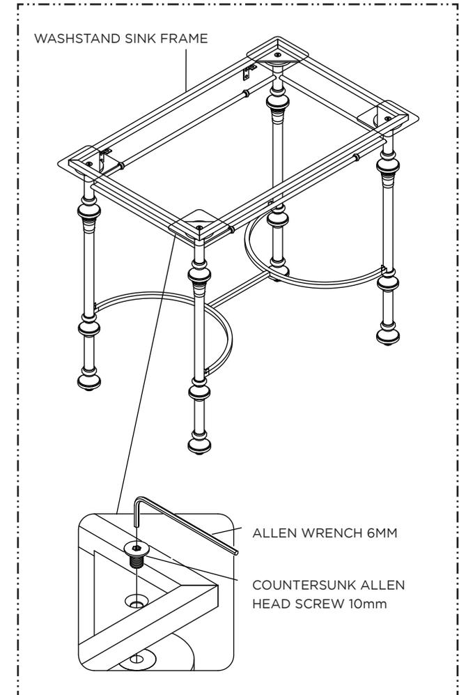
3. With the aid of two or more people place or sit the WASHSTAND SINK FRAME on the cavity on top of the LEGS and secure the FRAME with the COUNTERSUNK ALLEN HEAD SCREW. Tighten all the SCREWS with ALLEN WRENCH provided.
