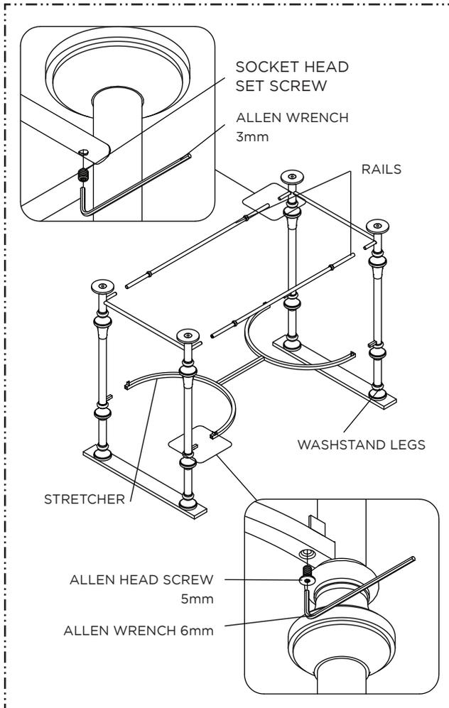
1. Arrange the WASHSTAND LEGS, RAILS, and STRETCHER with the hardware cavities facing inside. Set both legs in an upright position. Set the STRETCHER and the RAILS cavity on the LOCATOR of the leg. Secure the STRETCHER with the SOCKET FLAT HEAD SCREW and the RAILS with SOCKET HEAD SET SCREW. Repeat the procedure with the other leg.
