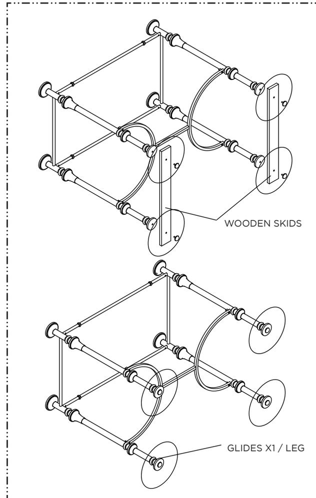
2. Remove the WOODEN SKIDS on the leg by loosening all the adjustable plastic glide. Re-install the adjustable GLIDES back to the LEG.
