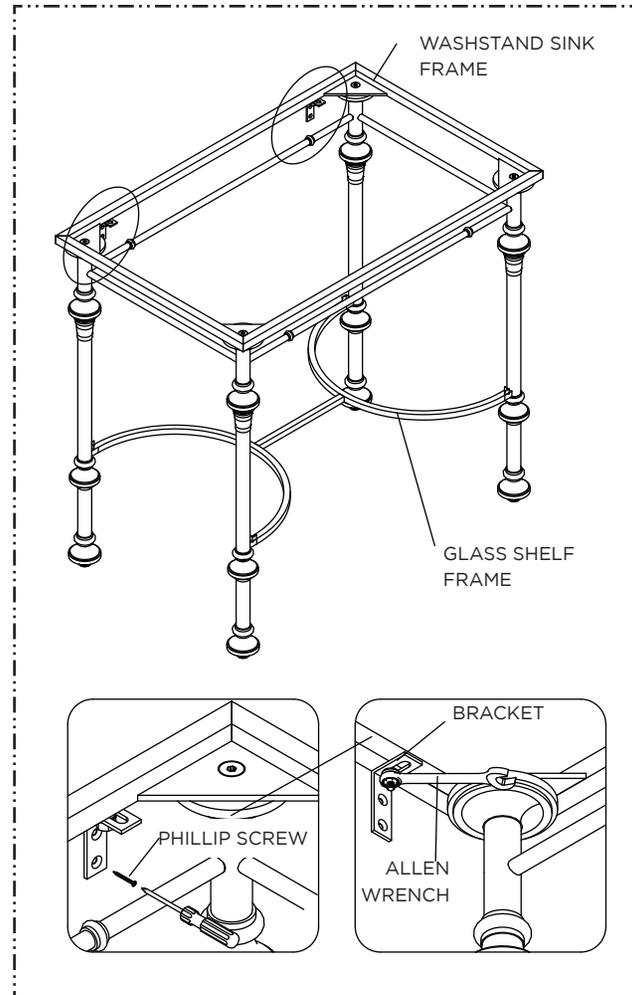
5. Slightly loosen the metal BRACKETS attached to the back of the WASHSTAND SINK FRAME. At your desired location, secure the WASHSTAND with the PHILLIP SCREW provided. Re-tighten the metal BRACKETS with the ALLEN WRENCH provided.
