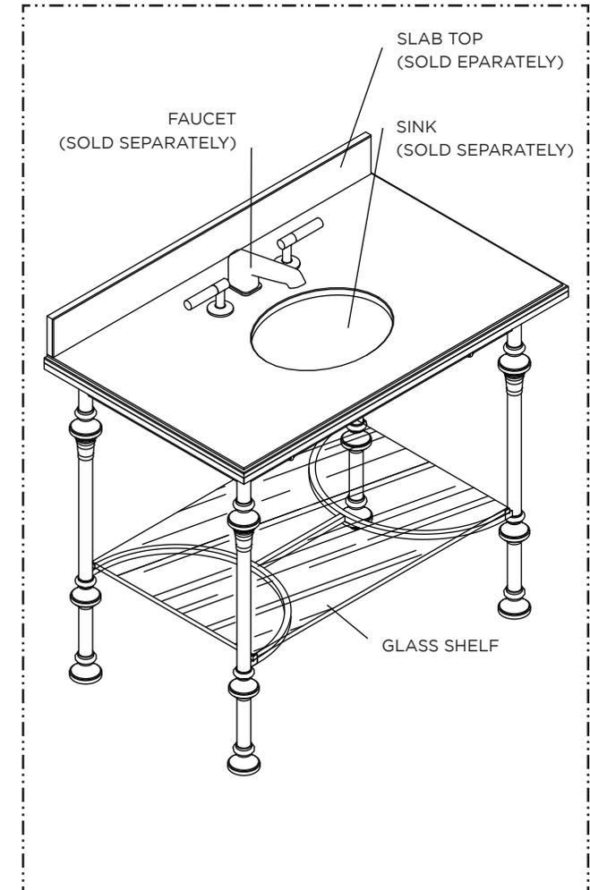
6. It is recommended to install the FAUCET and SINK to the SLAB TOP before setting it into the frame. The GLASS SHELF should be installed after plumbing is complete.
