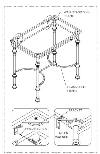
Slightly loosen the metal BRACKETS attached to the back of the WASHSTAND SINK FRAME. At your desired location, secure the WASHSTAND with the PHILLIP SCREW provided. Re-tighten the metal BRACKETS with the ALLEN WRENCH provided.
