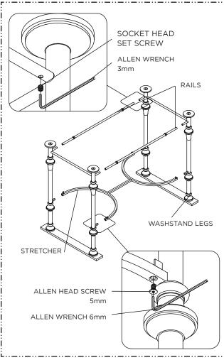
Arrange the WASHSTAND LEGS, RAILS, and STRETCHER with the hardware cavities facing inside. Set both legs in an upright position. Set the STRETCHER and the RAILS cavity on the LOCATOR of the leg. Secure the STRETCHER with the SOCKET FLAT HEAD SCREW and the RAILS with SOCKET HEAD SET SCREW. Repeat the procedure with the other leg.
