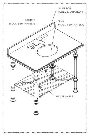
It is recommended to install the FAUCET and SINK to the SLAB TOP before setting it into the frame. The GLASS SHELF should be installed after plumbing is complete.
