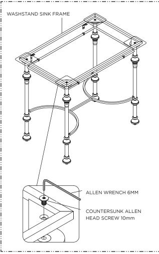
With the aid of two or more people place or sit the WASHSTAND SINK FRAME on the cavity on top of the LEGS and secure the FRAME with the COUNTERSUNK ALLEN HEAD SCREW. Tighten all the SCREWS with ALLEN WRENCH provided.
