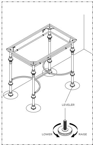
4. At the prepared location, pre-set the WASHSTAND against the wall, examine its alignment to see if leveling is necessary. If needed, slightly tilt the WASHSTAND and turn the LEVELERS clockwise to raise the fixture and counter-clockwise to lower it. Adjust all LEVELERS until the correct level is achieved.
