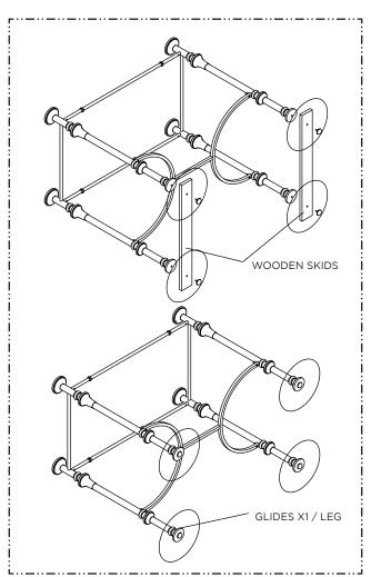
Remove the WOODEN SKIDS on the leg by loosening all the adjustable plastic glide. Re-install the adjustable GLIDES back to the LEG.
