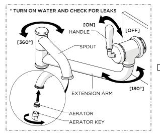
7. Turn on the water and operate the HANDLE to flush out any debris in the supply line and check for leaks then turn off water and re-install the AERATOR.
