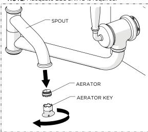
Unthread and remove the AERATOR from SPOUT using the AERATOR KEY provided.
