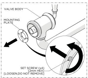
Loosen, but do NOT remove, the SET SCREWS (x4) using a 2mm HEX KEY then remove the MOUNTING PLATE from the VALVE BODY.
