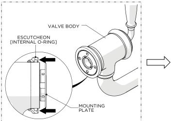
Slide the ESCUTCHEON against the VALVE BODY to expose the SET SCREWS.
