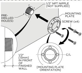
3. Ensure the NIPPLE (not supplied) protrudes 1/2" [13mm] in front of the finished wall then install the MONTING PLATE, in the proper orientation, using the SCREWS (x4) provided.
