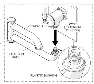
Remove the ARM to expose the POST with the external O-RINGS and PLASTIC BUSHING.
