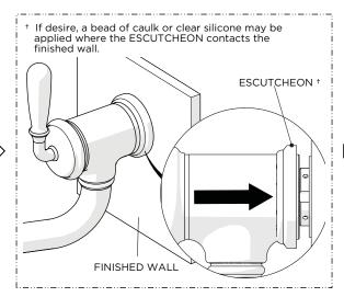
Slide the ESCUTCHEON down the VALVE BODY until it contacts the finished wall.
