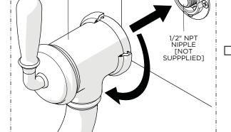
4. Thread and securely tighten the VALVE BODY onto the NIPPLE (not supplied).
