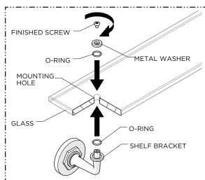
LOOSELY assemble both the SHELF BRACKETS onto the GLASS making sure to use the O-RINGS provided to prevent damage.
