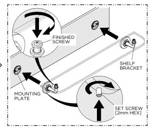
Place the BRACKETS over the MOUNTING PLATES and securely tighten the SET SCREWS and FINISHED SCREWS.
