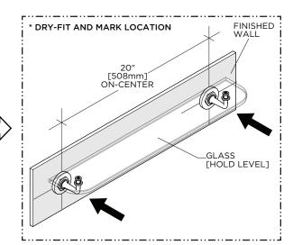
Dry-fit the product to the finished wall and mark the ideal location making sure to hold the product level.
