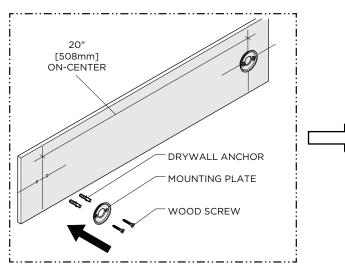
Using the previous marks as a reference, install the MOUNTING PLATES using the SCREWS and ANCHORS provided.
