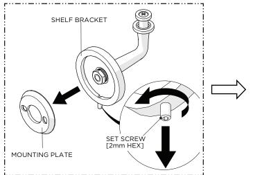
Loosen, but do NOT remove, the SET SCREW on the bottom of each SHELF BRACKET using a 2mm HEX KEY and remove the MOUNTING PLATES.
