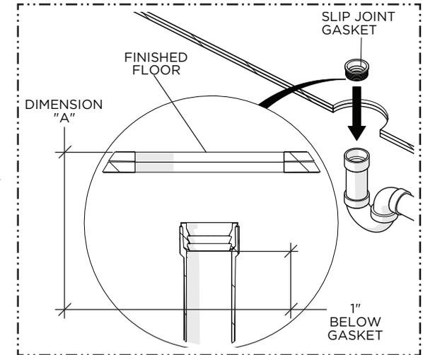
3. Insert the SLIP JOINT GASKET into the HUB then measure from the finished floor to 1" [25mm] past the bottom of the GASKET.
