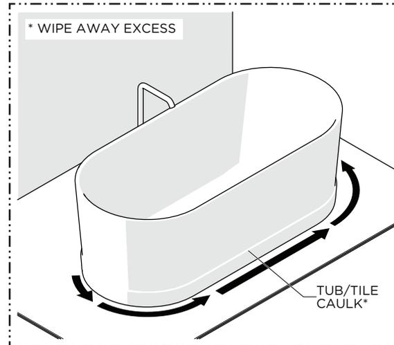
11. Run a bead of tub and tile caulk around the bottom edge of the BATHTUB where it meets the finished floor; wipe away any excess caulk with a wet paper towel.
