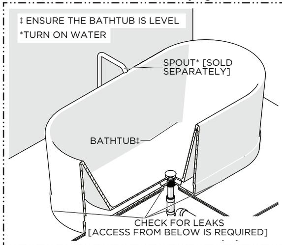
10. Verify the BATHTUB is level and, if needed, add shims then fill the BATHTUB until water enters the overflow hole. Drain the BATHTUB while inspecting all connections above and below the finished floor for leaks.
