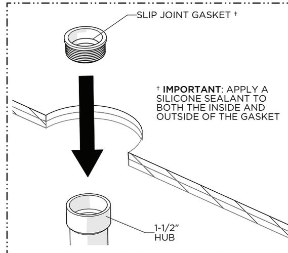
8. Apply a generous coating of silicone sealant to both the inside and outside of SLIP JOINT GASKET and insert the GASKET into the HUB.
