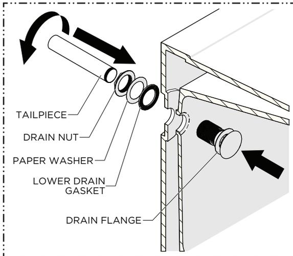
7. Apply a generous amount of putty or clear adhesive silicone to the underside of the DRAIN FLANGE and LOWER DRAIN GASKET then set the FLANGE into the TUB and attach the GASKET. Apply Teflon thread sealant to the FLANGE and TAILPIECE threads then attach the PAPER WASHER, DRAIN NUT, and TAILPIECE and securely tighten the NUT.
