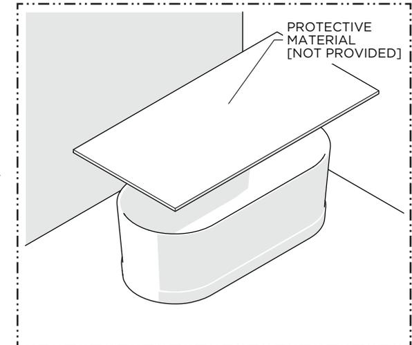
12. Cover the BATHTUB surface with a liner or other protective material (NOT PROVIDED) until construction is completed.
