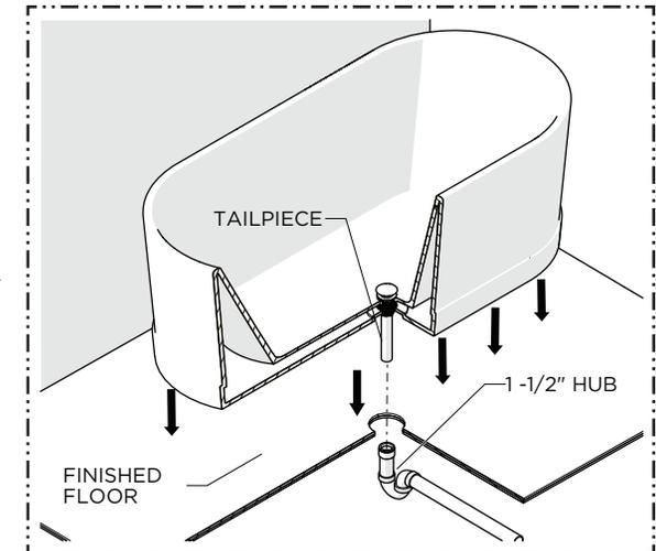
9. Move the BATHTUB into position and align the TAILPIECE with the HUB then carefully lower the BATHTUB until it fully rests on the finished floor.
