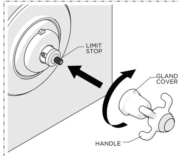
14. With the HANDLE in the desired orientation thread and securely tighten the GLAND COVER onto the LIMIT STOP.
