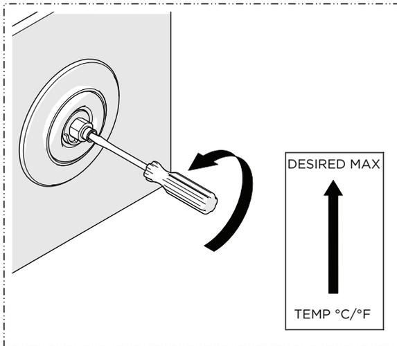
10. With water running, rotate the SQUARE TUBE to adjust the temperature to the **maximum** desired bathing temperature, verified with a thermometer then turn the water off.
