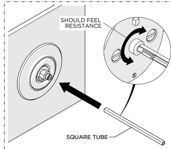
5. Insert the SQUARE TUBE into the TRIM NUT then, by feel, make sure it slides over the CARTRIDGE STEM and is fully seated.
