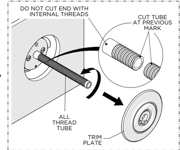
3. Remove the PLATE and TUBE then cut the TUBE at the previous mark.
