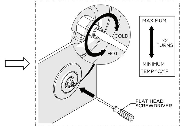
9. Insert a bladed screw driver into the SQUARE TUBE. Slowly rotate the TUBE clockwise to attain full cold then counterclockwise to attain full hot. It's approximately 2 complete rotations. Verify a full range of temperatures exists.
