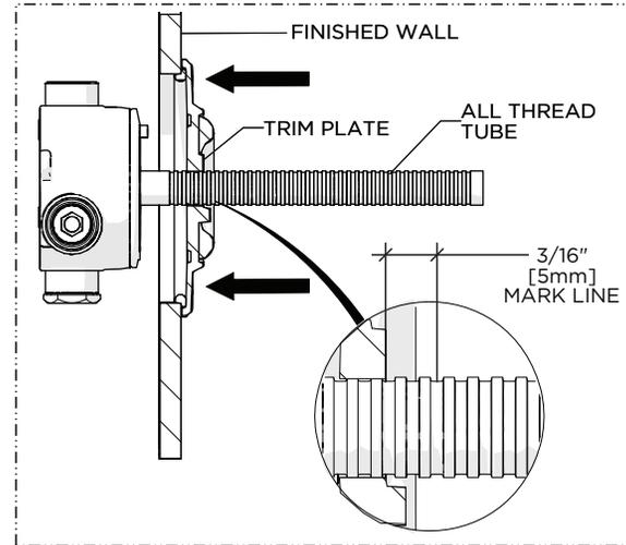
2. Firmly holding the TRIM PLATE against the finished wall, mark the TUBE 3/16" [5mm] beyond where it protrudes from the PLATE.
