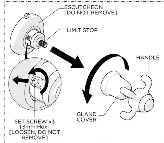
11. Unthread the GLAND COVER from the LIMIT STOP and pull the HANDLE off then loosen the SET SCREWS (x3) on the LIMIT STOP.
