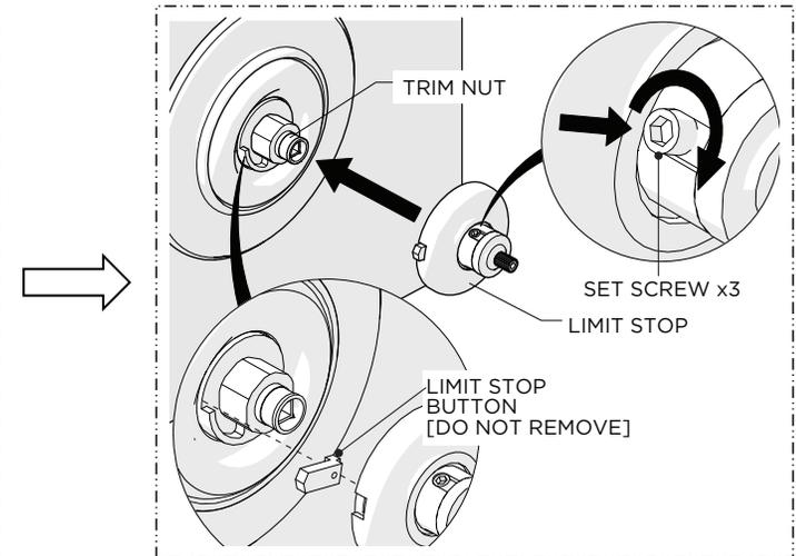
12. Place the LIMIT STOP onto the TRIM NUT making sure the LIMIT STOP BUTTON makes contact with the LIMIT STOP on the TRIM PLATE then securely tighten the SET SCREWS.
