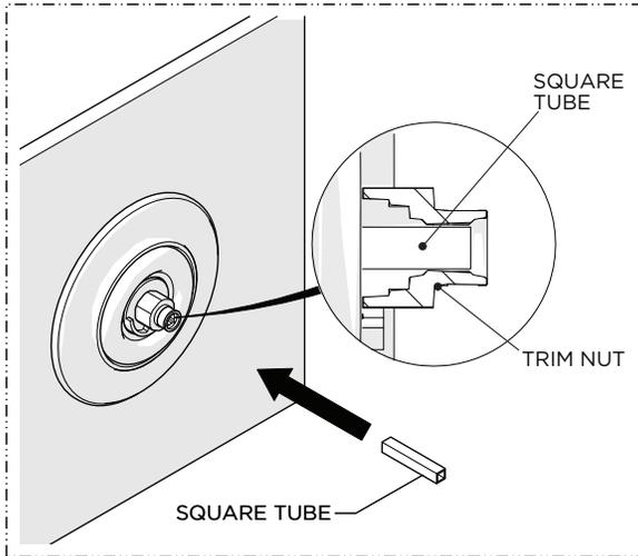
7. Re-insert the SQUARE TUBE back into the TRIM NUT making sure it is slight recessed.
