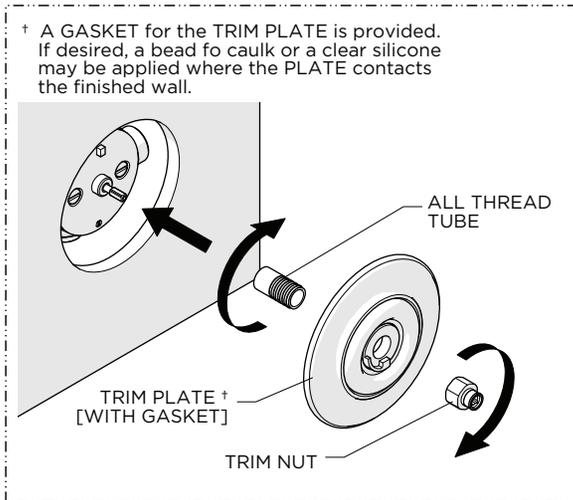
4. Thread the TUBE back onto the THERMOSTATIC VALVE and slide the PLATE over the TUBE then thread and securely tighten the TRIM NUT onto the TUBE to firmly hold the PLATE against the finished wall.
