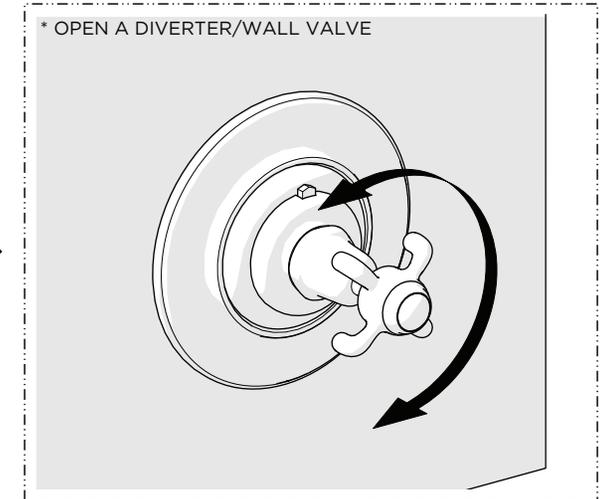
15. Open a diverter or wall valve (sold separately) and operate the HANDLE to ensure that it functions properly.
