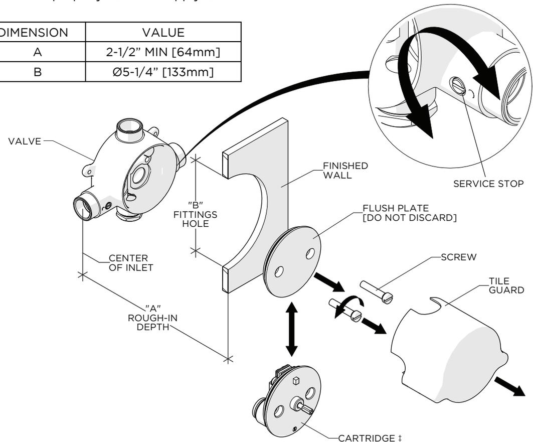
‡ **IMPORTANT:** The CARTRIDGE is packaged separately and provided with the VALVE.
