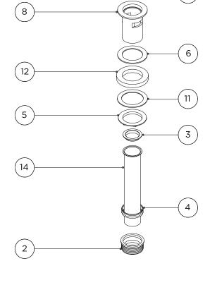
These guidelines have been prepared for the professional contractor to aid in the installation of: EMPIRE WASTE and OVERFLOW (Style # EMWO03) for Empire Tub (Style # EMBT01) & Colette Tub (Style #CBBT01)
