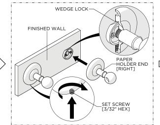
4. Place both PAPER HOLDER ENDS over the MOUNTING PLATES and securely tighten the SET SCREWS using a 3/32" HEX KEY.
