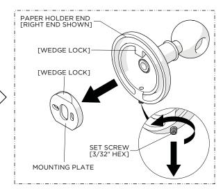
2. Loosen, but do <u>NOT</u> remove, the SET SCREW on the bottom of each PAPER HOLDER END using a 3/32" HEX KEY and remove the MOUNTING PLATES.
