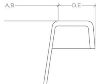
BATHING WELL (A,B) AND RIM (D,E) DIMENSIONS ARE TO THE TOP OF RADIUS AS SHOWN.
