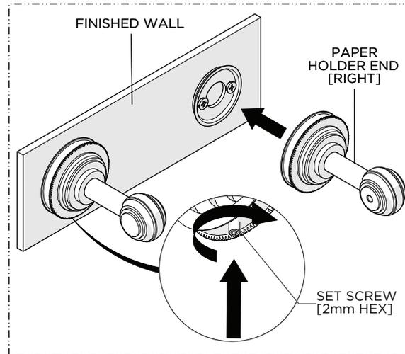
4. Place both PAPER HOLDER ENDS over the MOUNTING PLATES and securely tighten the SET SCREWS using a 2mm HEX KEY.
