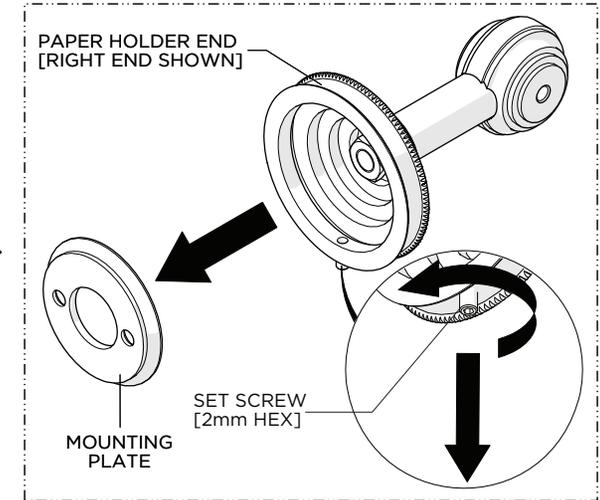
2. Loosen, but do **NOT** remove, the SET SCREW on the bottom of each PAPER HOLDER END using a 2mm HEX KEY and remove the MOUNTING PLATES.
