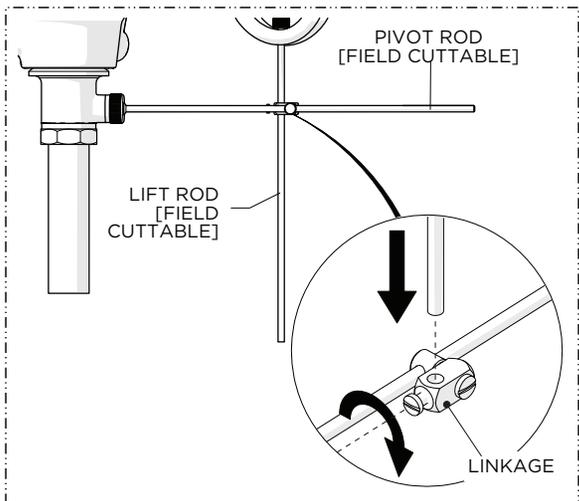
22. Connect the LIFT ROD to the PIVOT ROD using the LINKAGE provided.
