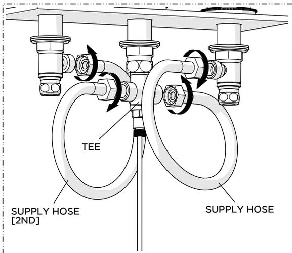
16. Connect the SIDEBODIES to the TEE using the SUPPLY HOSES provided. Securely tighten the HOSES and ensure they are not pinched/kinked.
