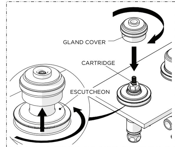
12. Thread the GLAND COVER onto the CARTRIDGE until it stops then unthread the ESCUTCHEON until it contacts the GLAND COVER.
