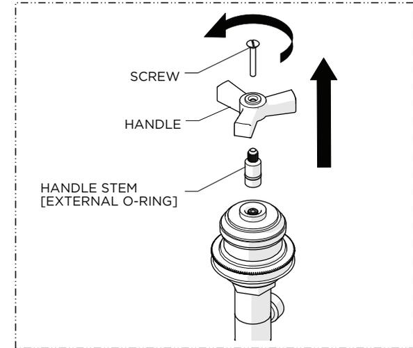
9. Unthread the SCREW then remove the HANDLE and HANDLE STEM.
