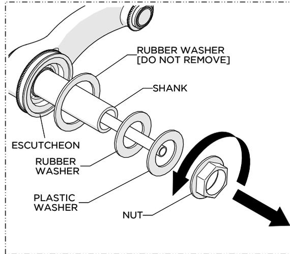
2. Unthread and remove the NUT and lower deck WASHERS from the SHANK.
