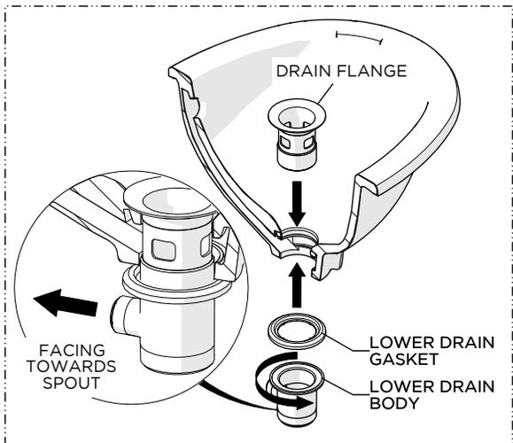
19. Set the DRAIN FLANGE into the lavatory (sold separately) using putty or a clear silicone and attach the LOWER DRAIN GASKET then securely tighten the LOWER DRAIN BODY onto the FLANGE.
