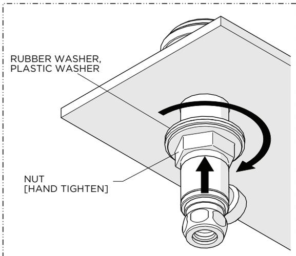
13. Hand-tighten the NUT against the underside of the mounting surface.
