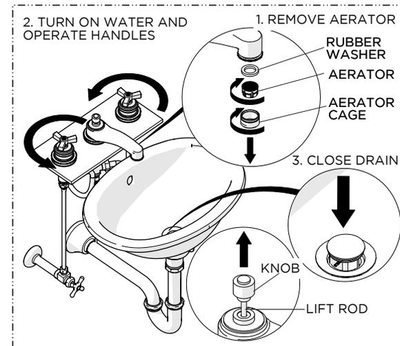
24. Remove the AERATOR, turn on the water to flush out the supply lines, inspect all connections for leaks, and close the DRAIN to ensure it functions properly. Turn off and drain the water then re-install the AERATOR.
