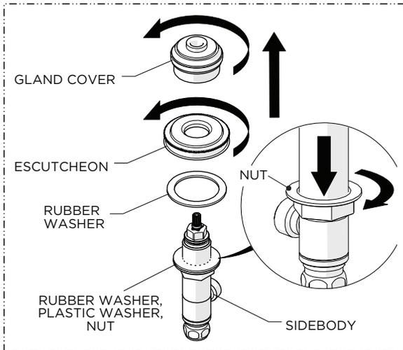
10. Remove the GLAND COVER, ESCUTCHEON and RUBBER WASHER from the SIDEBODY then fully thread the NUT down.
