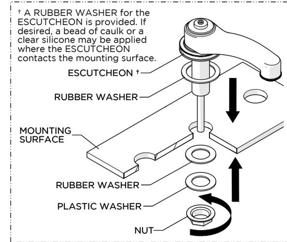
3. Insert the SHANK through the hole on the mounting surface making sure the RUBBER WASHER is beneath the SPOUT then reattach the lower deck WASHERS and securely tighten the NUT.
