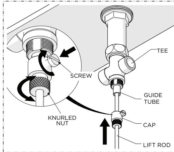
8. Slide the CAP up the LIFT ROD and onto the GUIDE TUBE then securely tighten the SCREW.
