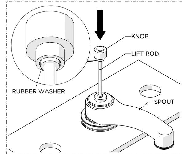
6. Insert the LIFT ROD into the top of the SPOUT making sure the RUBBER WASHER is beneath the KNOB.
