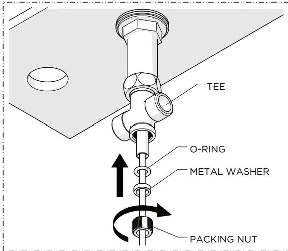
7. Insert the O-RING and METAL WASHER into the base of the TEE then insert and securely tighten the PACKING NUT.
