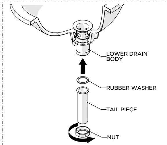
20. Re-attach the TAILPIECE then securely tighten the NUT onto the LOWER DRAIN BODY making sure to use the RUBBER WASHER provided.
