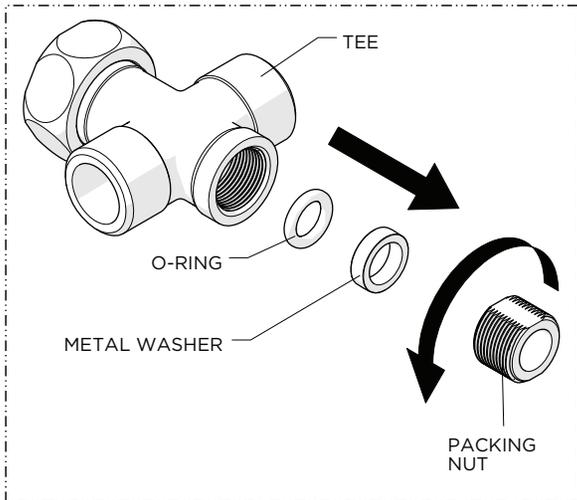
4. Remove the PACKING NUT, METAL WASHER and O-RING from the TEE to prevent the GUIDE TUBE in the SPOUT from damaging the O-RING.
