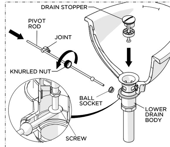
21. Making sure the BALL SOCKET is in place, insert the PIVOT ROD into the DRAIN BODY and securely tighten the NUT then insert the STOPPER into the FLANGE making sure the SCREW rests on top of the PIVOT ROD. Adjust the SCREW if needed.
