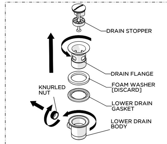
18. Unthread and remove the LOWER DRAIN BODY, LOWER DRAIN GASKET, and the DRAIN STOPPER from the DRAIN FLANGE. Unthread and remove the KNURLED NUT from the LOWER DRAIN BODY.
