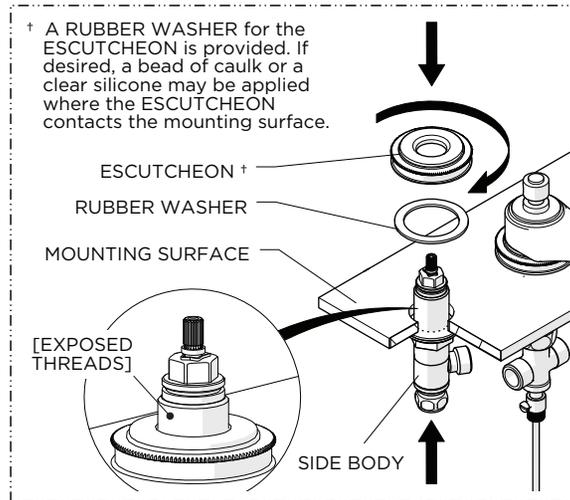
11. Using the RUBBER WASHER provided, thread the ESCUTCHEON back onto the SIDEBODY then let it rest on the mounting surface.
