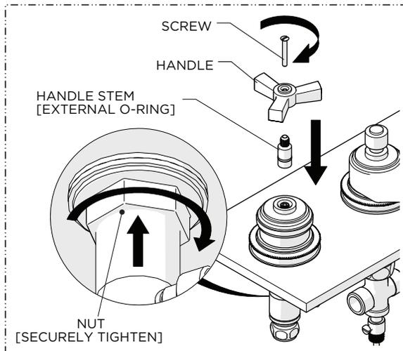
14. Fully insert the HANDLE STEM into the GLAND COVER and place the HANDLE onto the STEM then thread and securely tighten the SCREW. Ensure the HANDLE is in the desired orientation then securely tighten the NUT.
