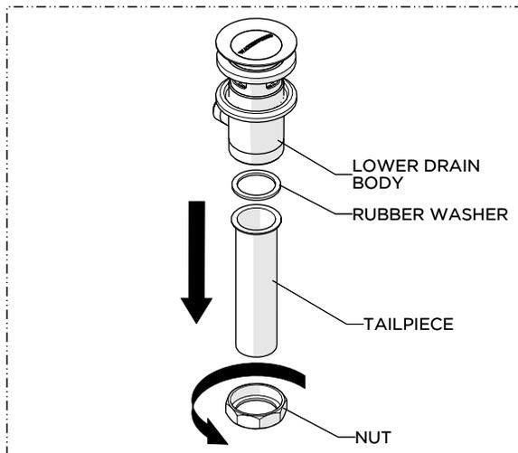
17. Unthread and remove the NUT, TAILPIECE, and the RUBBER WASHER from the LOWER DRAIN BODY.
