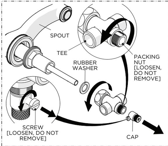
1. Loosen but do NOT remove the SCREW on the CAP then remove the CAP. Loosen but do NOT remove the PACKING NUT at the base of the TEE then remove the TEE and RUBBER WASHER from the SHANK.
