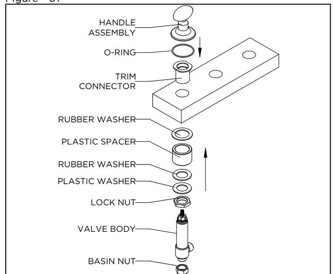
These guidelines have been prepared for the professional contractor to aid in the installation of: OPUS LOW PROFILE THREE HOLE LAVATORY FAUCET WITH CRYSTAL EGG HANDLES (STYLE# OPLS02), METAL LEVER HANDLES (STYLE # OPLS05), AND CRYSTAL LEVER HANDLES (STYLE# OPLS06)
