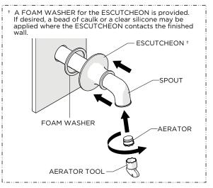
6. Re-install the AERATOR then slide the ESCUTCHEON down the SPOUT until it contacts the finished wall.
