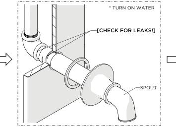
5. Turn on the water and a diverter/wall valve (sold separately) to flush out any debris in the supply line and inspect all connections for leaks then turn the water off.
