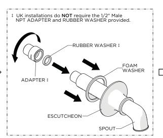
2. Slide the ESCUTCHEON onto the SPOUT, making sure to use the FOAM WASHER provided, then thread the 1/2" NPT ADAPTER ‡ onto the SPOUT using the RUBBER WASHER provided.
