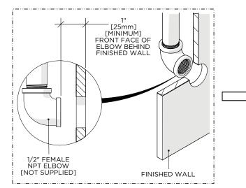
1. Ensure the ELBOW (not supplied) is properly roughed-in to the appropriate depth.
