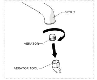
4. Using the TOOL provided, remove the AERATOR.
