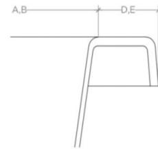
BATHING WELL (A,B) AND RIM (D,E) DIMENSIONS ARE TO THE TOP OF RADIUS AS SHOWN.
