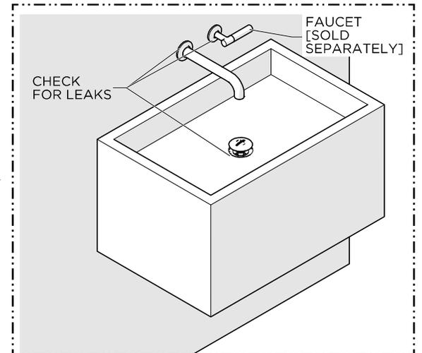
6. Turn on the water and operate the drain and faucet [sold separately] to ensure proper operation. Check all connections for leaks. If desired, a bead of caulk or clear silicone may be applied where the SINK contacts the finished wall.
