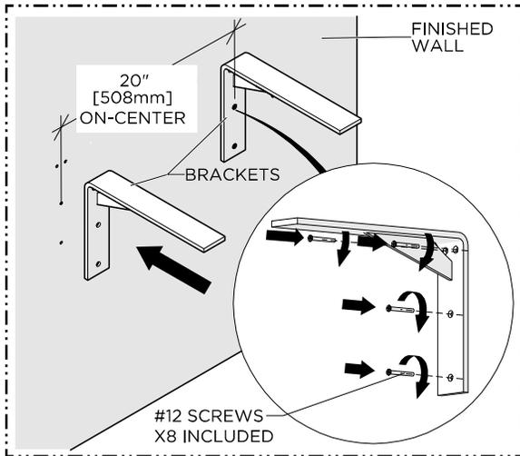
1. Dry fit the BRACKETS to the FINISHED WALL and mark the location of the mounting holes. Make sure to hold the BRACKETS level. Drill pilot holes for the #12 WOOD SCREWS provided. Secure the BRACKETS using the #12 WOOD SCREWS.
