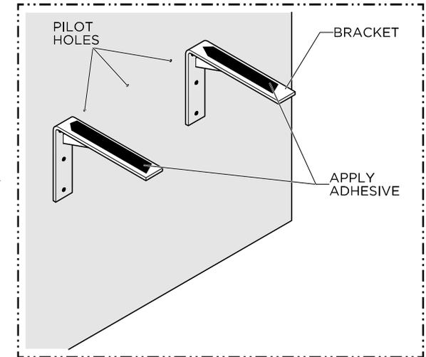
3. Apply adhesive silicone to the top surfaces of the BRACKETS.
