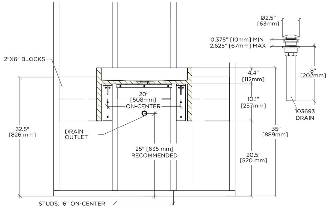
**Note:** This blocking scheme installs the sink top 35" from the floor.
