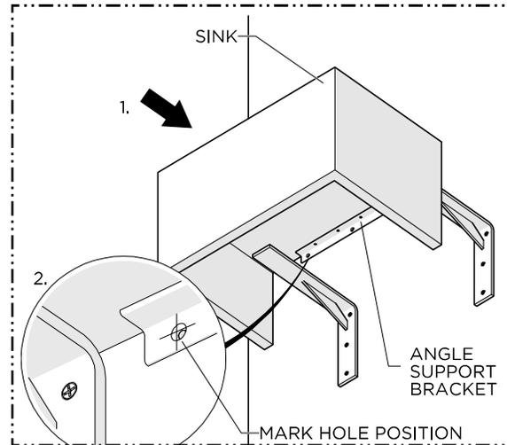
2. Dry fit the SINK with ANGLE SUPPORT BRACKET ensuring it is level and re-adjust or shim (not included) if necessary. Mark the three holes locations for the ANGLE SUPPORT BRACKET. Remove the SINK and drill pilot holes for #12 WOOD SCREWS.
