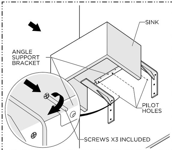
4. Place the SINK on top of the BRACKETS and push it against the wall making sure the silicone does not wipe off. Remove any excess silicone around the SINK. Fasten the ANGLE SUPPORT BRACKET with the #12 WOOD SCREWS provided.
