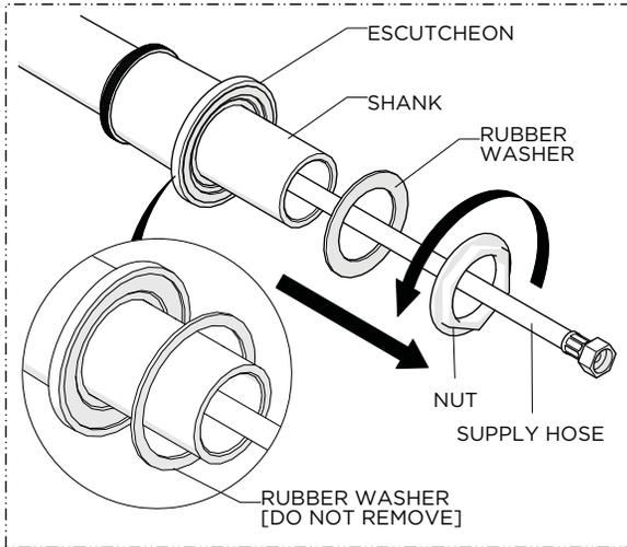
1. Unthread and remove the NUT and RUBBER WASHER from the SHANK.
