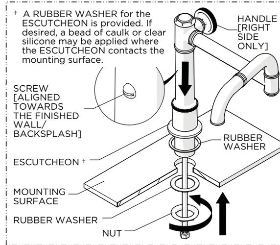
2. Insert the SPOUT through the hole on the mounting surface making sure the SCREW on the SPOUT COLUMN is aligned towards the finished wall then using the RUBBER WASHER provided and securely tighten the NUT onto the SHANK.
