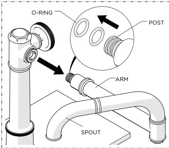
2. Remove the ARM to expose the POST and access the O-RINGS.
