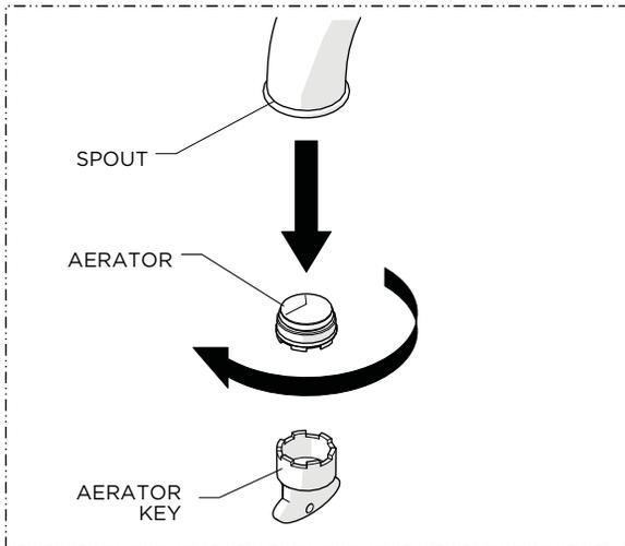
4. Using the TOOL provided, remove the AERATOR.
