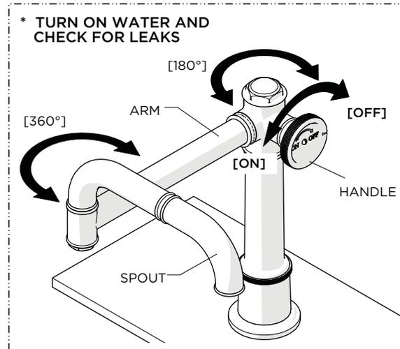
5. Turn on water and operate HANDLE and SPOUT to ensure they function properly and to flush out any debris in the supply line then check all connections for leaks and turn off the water.
