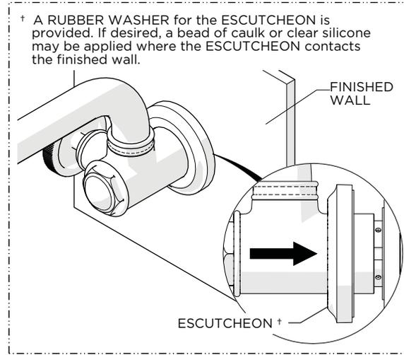
8. Slide the ESCUTCHEON down the VALVE BODY until it contacts the finished wall.
