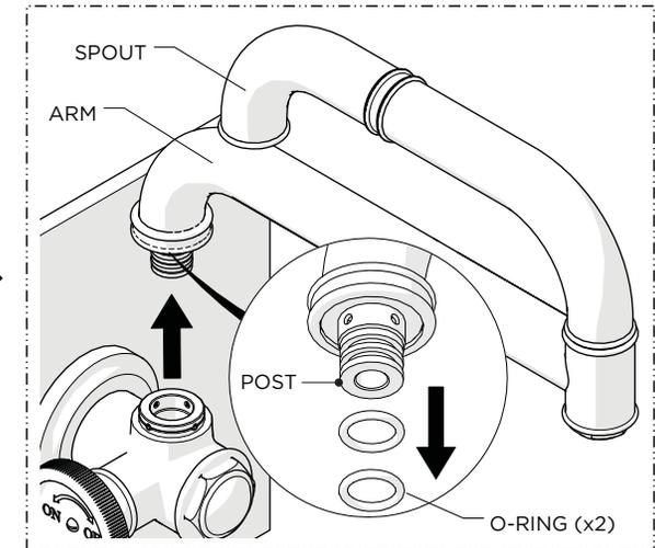
2. Remove the ARM to expose the POST and access the O-RINGS.
