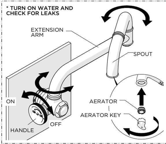
7. Turn on the water and operate the HANDLE to flush out any debris in the supply line and check for leaks then turn off water and re-install the AERATOR.
