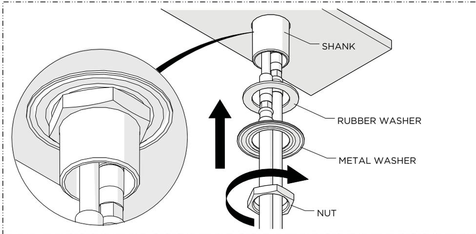
4. Re-attach the RUBBER and METAL WASHERS then thread and securely tighten the NUT onto the SHANK.
