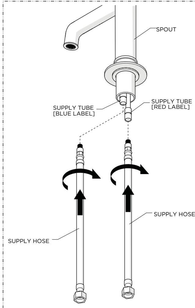
2. Thread and securely tighten the SUPPLY HOSES onto the SUPPLY TUBES installed on the SPOUT.
