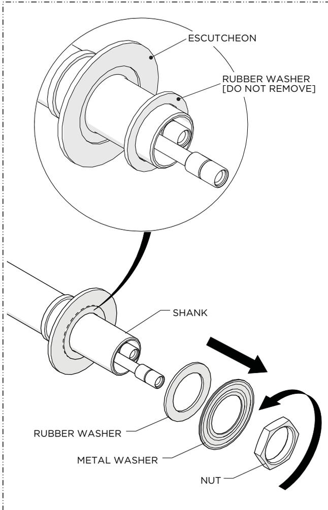
1. Unthread and remove the NUT from the SHANK then remove the METAL and RUBBER WASHERS
