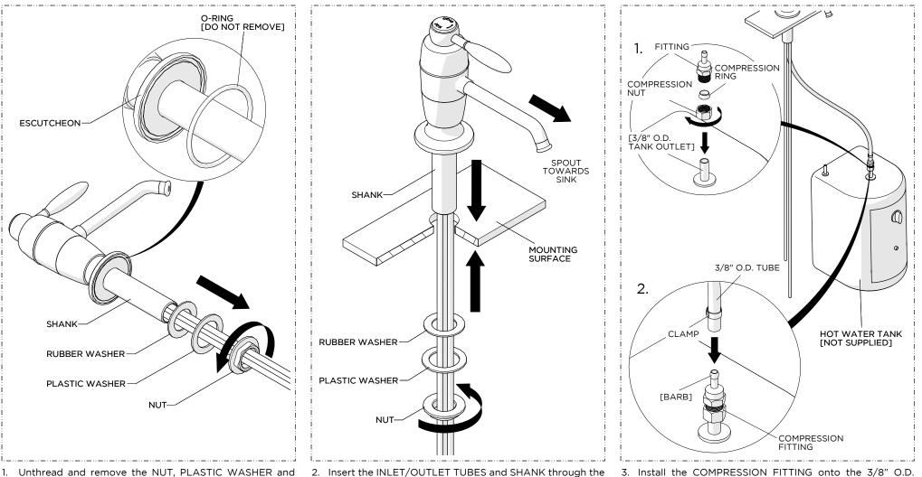
1. Unthread and remove the NUT, PLASTIC WASHER and RUBBER WASHER from the SHANK.
