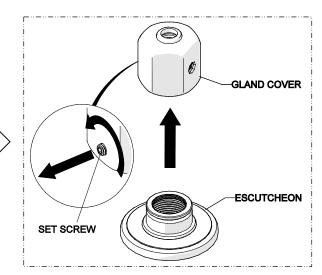
Unthread, but do not fully remove the SET SCREW, then detach the GLAND COVER from the ESCUTCHEON.
