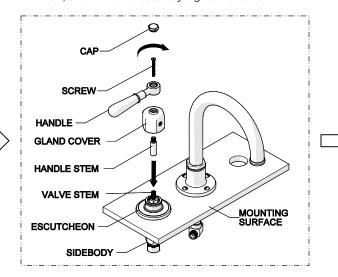
5. Place the HANDLE STEM on the VALVE STEM, then place the GLAND COVER onto the ESCUTCHEON, making sure it is fully seated. Install the HANDLE on the HANDLE STEM in the desired orientation and securely tighten the SCREW, then insert the CAP into the HANDLE. DO NOT tighten SET SCREW at this time.
