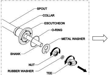
Remove the TEE, NUT and lower deck WASHERS from the SPOUT SHANK. Do NOT remove the O-RING from the ESCUTHCEON.
