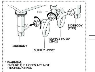
8. Connect the SIDEBODIES to the TEE using the SUPPLY HOSES provided. Securely tighten the HOSES and ensure they are not pinched/kinked.
