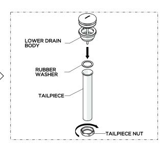
Remove the TAILPIECE from the LOWER DRAIN BODY.
