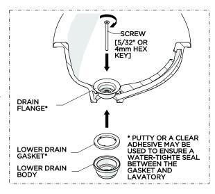
12. Re-install the LOWER DRAIN BODY making sure to use the GASKET provided. Ensure the GASKET makes a full seal on the underside of the lavatory then securely tighten the SCREW.
