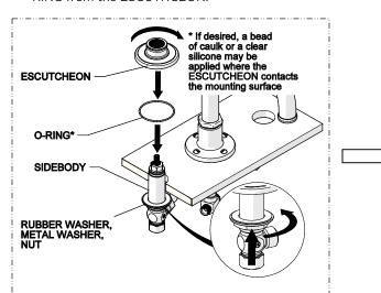
4. Thread the ESCUTCHEON back onto the SIDEBODY until it stops and let it rest on the mounting surface. Hand tighten the NUT against the underside of the mounting surface.
