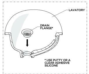
Set the DRAIN FLANGE in the lavatory [SOLD SEPARATELY] using putty or a clear adhesive silicone.
