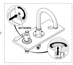
Ensure the HANDLE is in the desired orientation then securely tighten the NUT on the SIDE BODY. Align the GLAND COVER as shown then securely tighten the SET SCREW.
