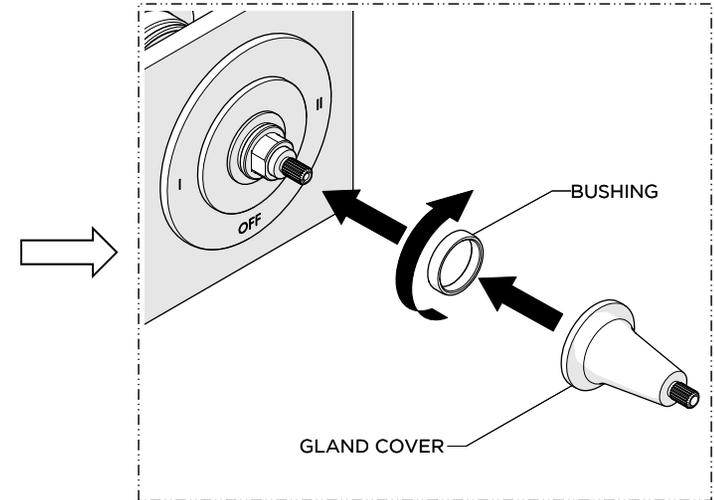
9. Thread the PLASTIC BUSHING onto the TRIM NUT then place the GLAND COVER over the TRIM NUT making sure it is fully seated.
