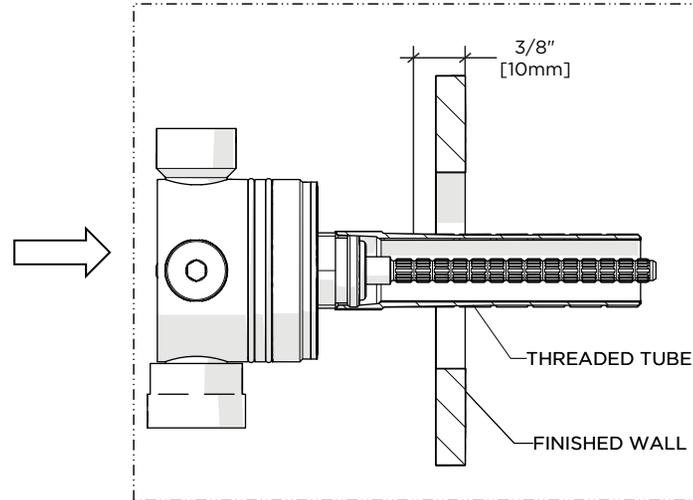
2. Mark the THREADED TUBE 3/8" [10mm] behind the finished wall.
