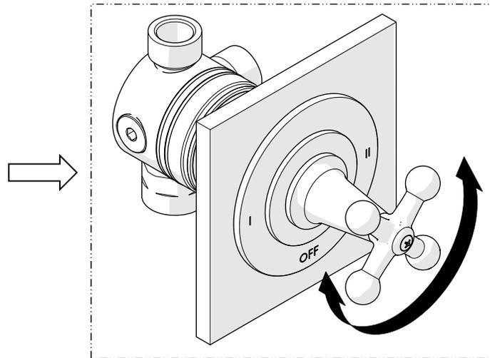
11. Turn on the water and operate the HANDLE to ensure it is functioning properly.
