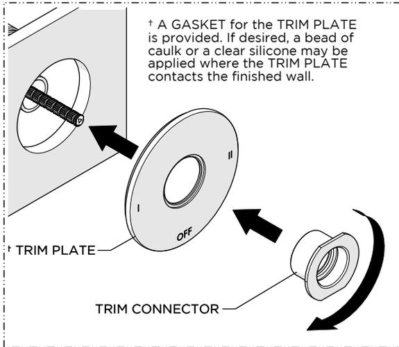
7. Hold the TRIM PLATE against the finished wall then thread and securely tighten the TRIM CONNECTOR.
