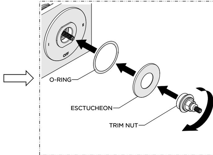
8. Hold the ESCUTCHEON against the TRIM PLATE, making sure to include the O-RING, then thread and securely tighten the TRIM NUT into the TRIM CONNECTOR.
