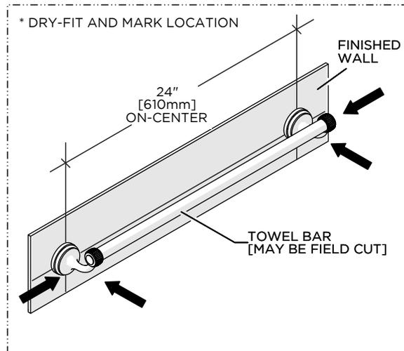
1. Dry-fit the product to the finished wall and mark the ideal location making sure to hold the product level.
