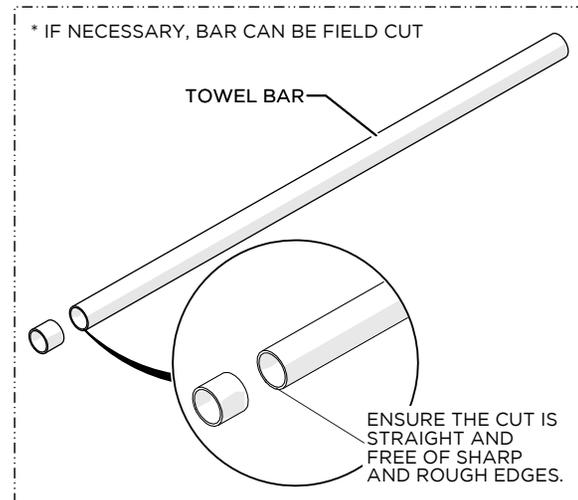
**OPTIONAL:** If necessary, the BAR may be cut. Ensure the cut is straight and free of sharp and rough edges.
