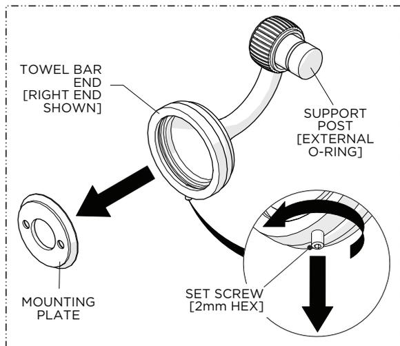
3. Loosen, but do **NOT** remove, the SET SCREW on the bottom of each TOWEL BAR END using a 2mm HEX KEY and remove the MOUNTING PLATES.
