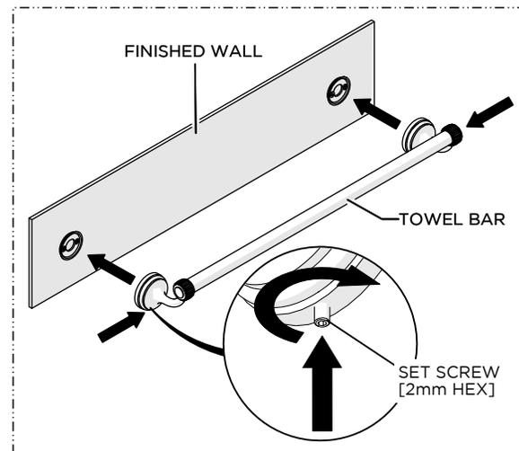
5. Holding the ENDS and BAR together, place both ENDS over the MOUNTING PLATES and securely tighten the SET SCREWS.
