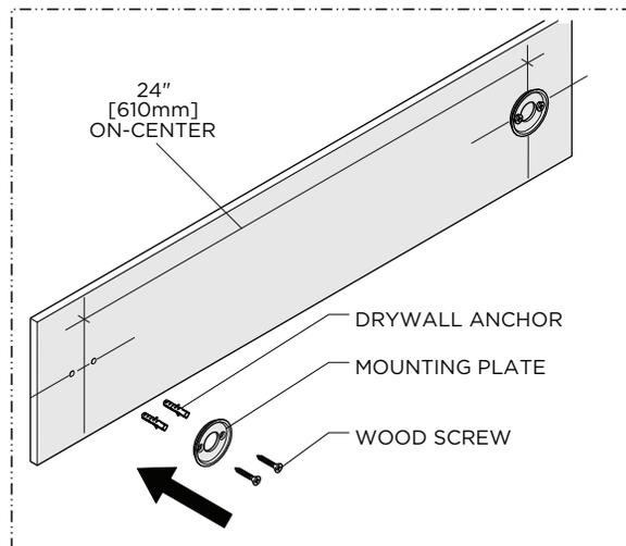
4. Using the previous marks as a reference, install the MOUNTING PLATES using the SCREWS and ANCHORS provided.
