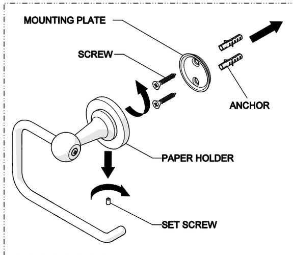
1. Unthread the SET SCREW and remove the MOUNTING PLATE, SCREWS and ANCHORS from PAPER HOLDER.
