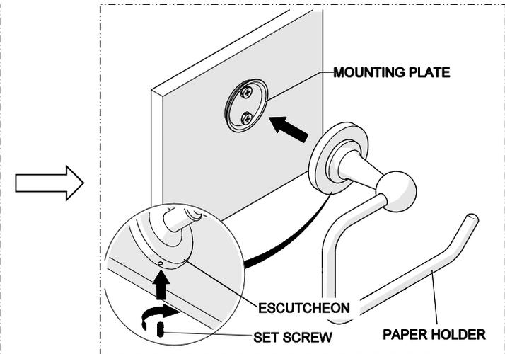
3. Place the PAPER HOLDER over the MOUNTING PLATE then thread and securely tighten the SET SCREW into the ESCUTCHEON.
