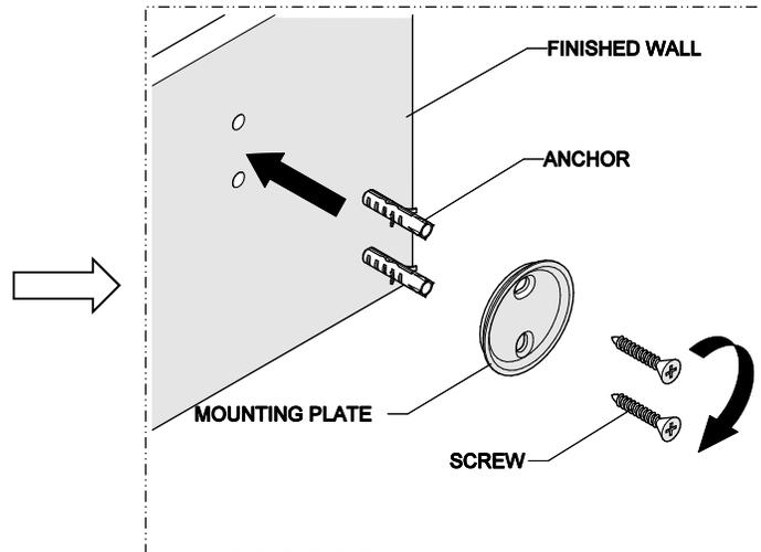
2. Secure the MOUNTING PLATE onto the finished wall using the SCREWS provided.
