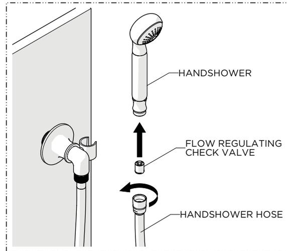
5. Thread and securely tighten the conical end of the HOSE to the HANDSHOWER.
