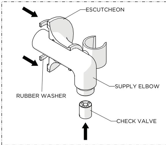
1. Slide the ESCUTCHEON and RUBBER WASHER onto the SUPPLY ELBOW.
