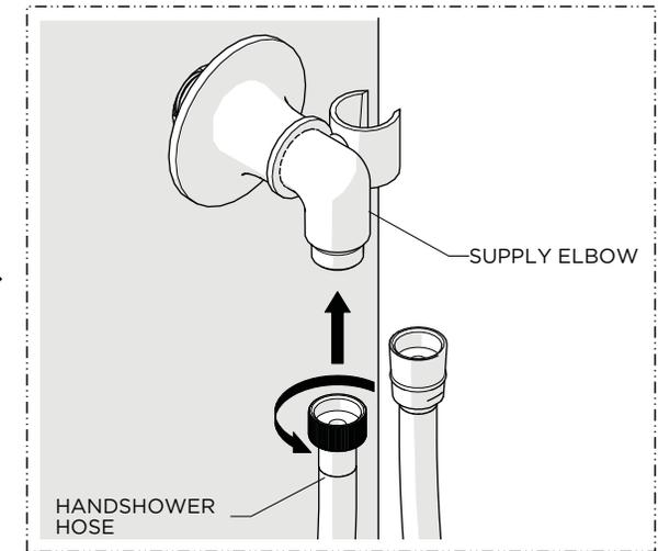
3. Thread and securely tighten the knurled end of the HOSE to the ELBOW.
