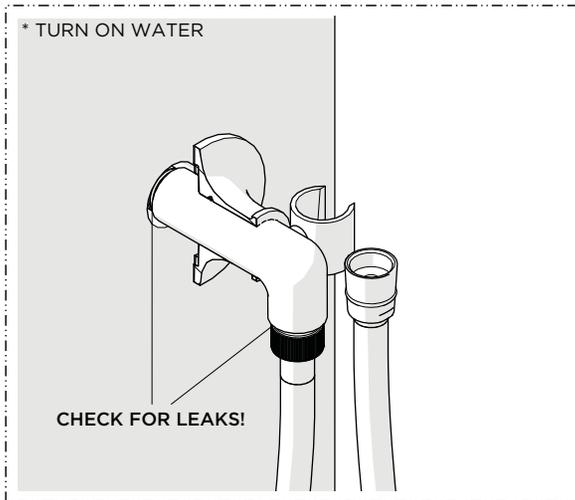
4. Turn on the water and a diverter/wall valve (sold separately) to flush out any debris in the supply line and inspect all connections for leaks then turn the water off.
