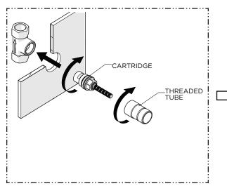
Thread and securely tighten the CARTRIDGE back into the VALVE then thread the THREADED TUBE back onto the CARTRIDGE until it stops
