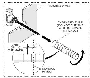
2. Remove the THREADED TUBE then cut it 7/16" [11mm] behind the previous mark.
