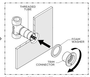
6. Using the FOAM WASHER provided, thread the TRIM CONNECTOR onto the THREADED TUBE.
