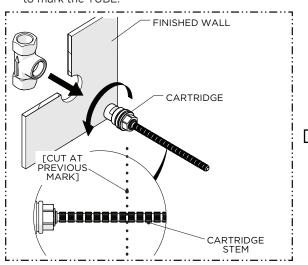
4. Remove the CARTRIDGE using a 21/32" [17mm] shower valve socket wrench (not supplied) then cut the CARTRIDGE STEM at the previous mark.
