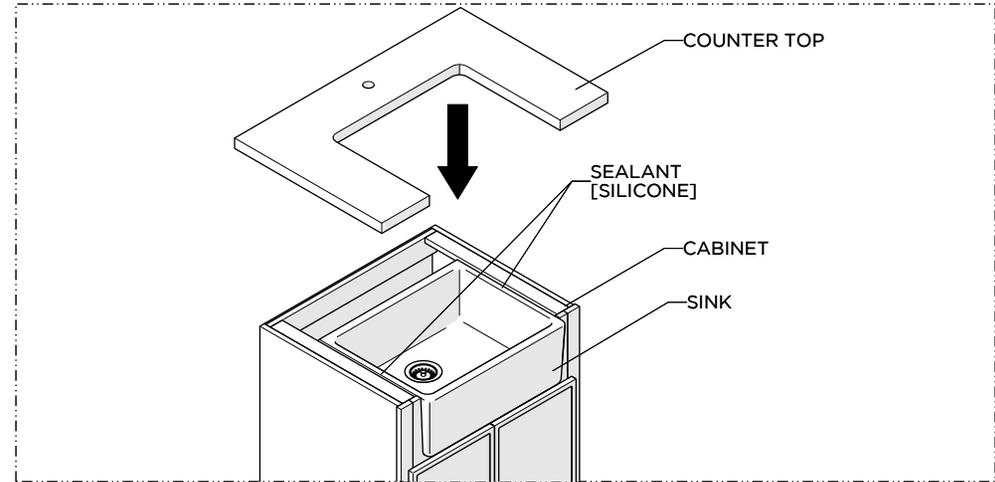
10. Apply a bead of silicone sealant to the back and sides of the SINK then place the countertop on top of the cabinets.
