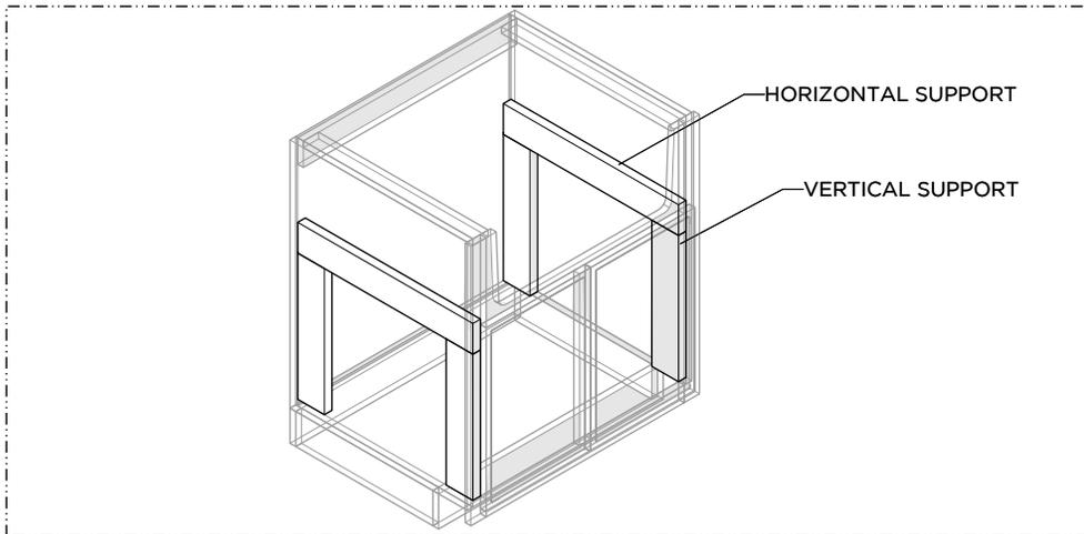
3. Using adequate support framing material, install a support frame inside the **CABINET** that will securely support the weight of the **SINK**. **EXAMPLE:** A support frame may consist of 2 horizontal supports, 4 vertical supports, and a sheet of 3/4" plywood.
