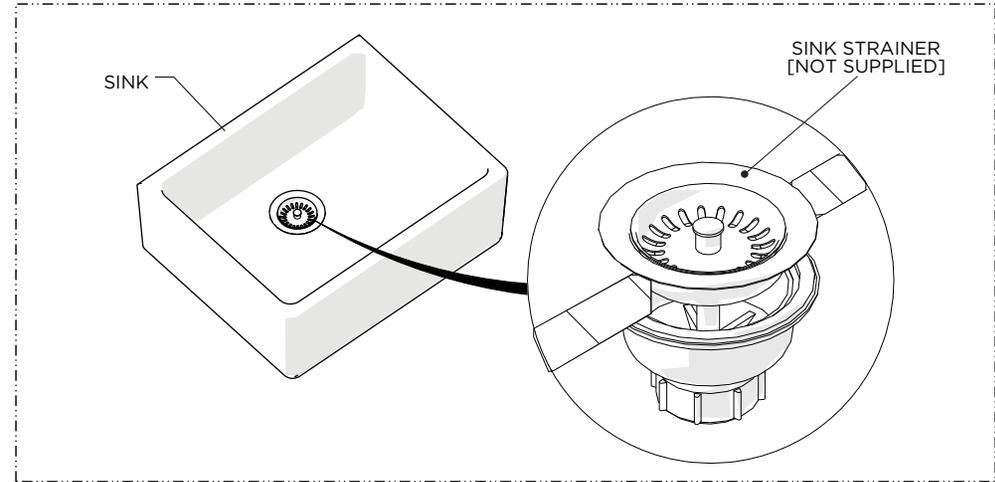
6. Install the strainer onto the SINK, per the manufacturer's instructions.
