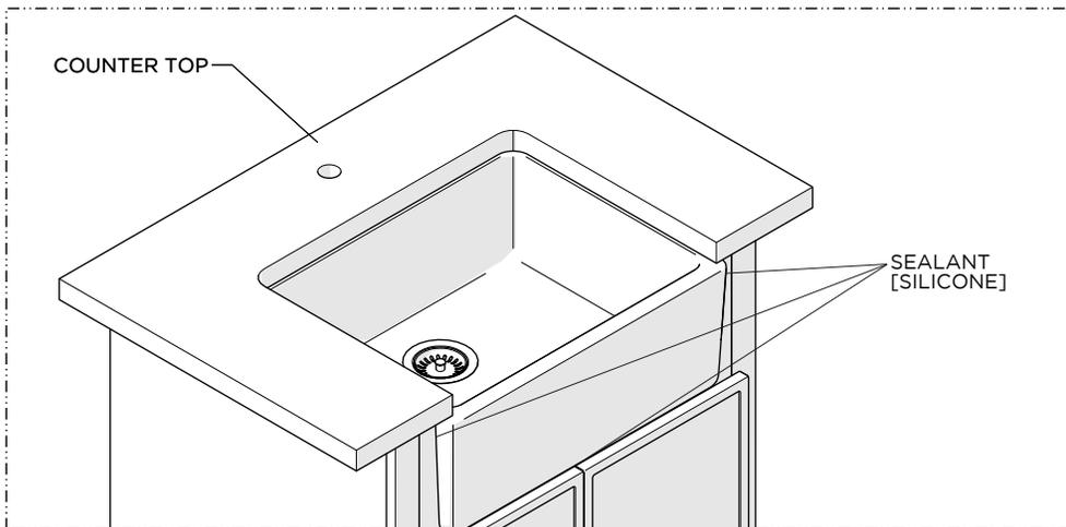
11. Apply a bead of silicone sealant where the SINK contacts the countertop and cabinet surfaces. Remove any excess sealant.
