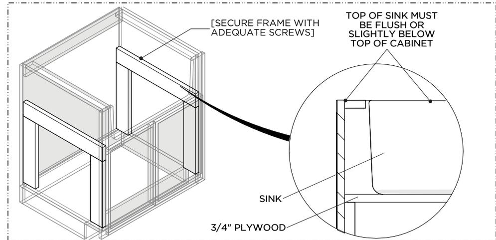
4. Ensure that the supports are secured using **SCREWS** (not provided) and level.
